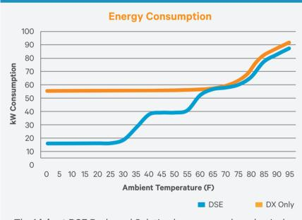
The **Liebert DSE** Packaged Solution has an annual mechanical PUE of under 1.20. Its advanced Liebert iCOM™ controls automatically transition operating modes to maximize annual economization hours, compared to units running only in DX (direct expansion) mode. Additionally, low air leakage compared to heat wheels means less capacity is required for makeup air and conditioning.
