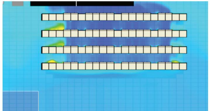
*The Red Sky supercomputer uses a laminar airflow configuration, with perforated floor tiles required only in the first row of racks. The 72-degree air expelled from the Liebert XDR cooling doors feeds into the front of the next rack, and cascades through each rack row.*
