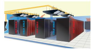
The Liebert XDO systems work extremely well with the "hot aisle-cold aisle" approach.
