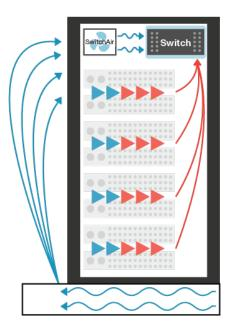
SwitchAir products direct cool air to the network switches, significantly lowering operating temperatures.
