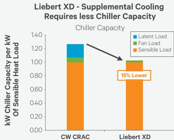
One of the major areas of savings identified with the use of Liebert XD equipment is the fact that the chiller plant size can be reduced. This is because the chiller typically is sized for the total gross capacity of the raised-floor cooling units. The 65% lower fan load of the Liebert XD System modules and the fact they are 100% sensible easily results in a capital chiller size savings of 15% or more.
