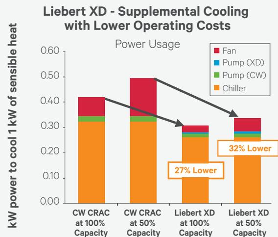
The smaller chiller plant and lower fan load result in significant energy savings as well. A 27% energy savings is very conservative.
