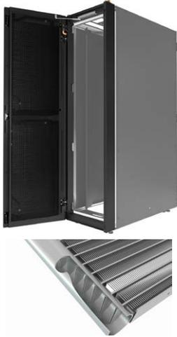
The Liebert XDR design uses the server fans within the protected rack to provide airflow through the unit. The microchannel coil heat exchanger cools the air and returns it to room at close to the same temperature as the air entering the rack.
