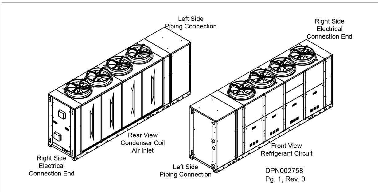
Figure 3.11 Isometric views FG0080 / FB0110 without buffer tank
