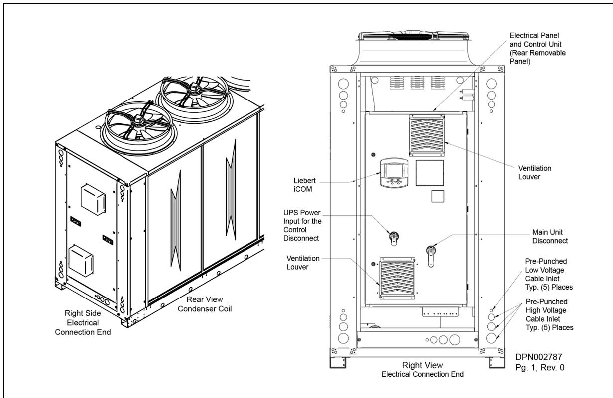
Figure 3.14 High-voltage, low-voltage electrical field connection locations and cable entry points
