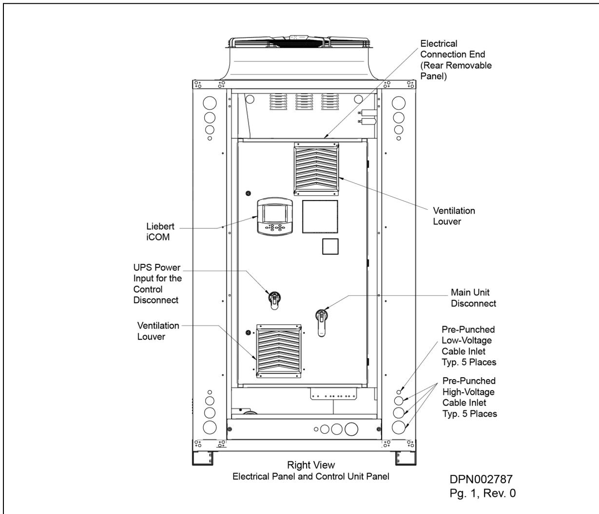
Figure 3.16 Suggested internal pathways for high-voltage, low-voltage electrical wiring
