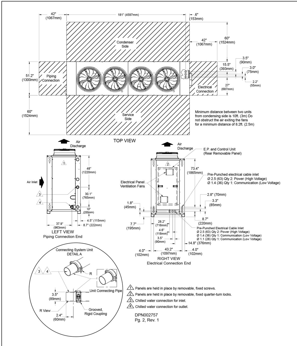
Figure 3.3 Dimensions, fan sizes and piping connections for Liebert HPC-S model FG0052 with buffer tank
