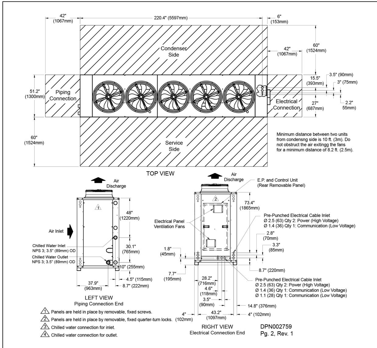
Figure 3.7 Dimensions, fan sizes and piping connections for Liebert HPC-S models FG0080 and FB0 110 with integral free-cooling and buffer tank
