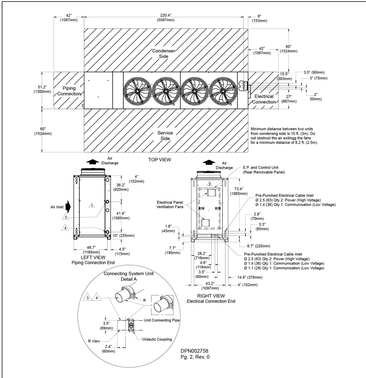
Figure 3.5 Dimensions, fan sizes and piping connections for Liebert HPC-S models FG0080 and FB0110, no buffer tank
