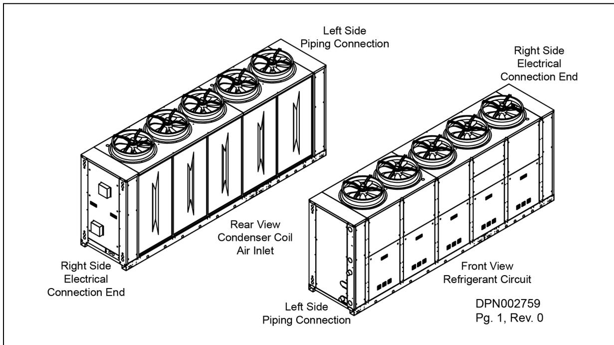
Figure 3.12 Isometric views FG0080 / FB0110 with buffer tank
