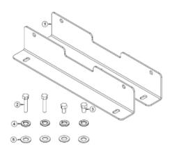
Bolt down kit is an optional part which is used to prevent racks from tipping over during installation or maintenance of equipment. It also secures an assembled rack during transport.
