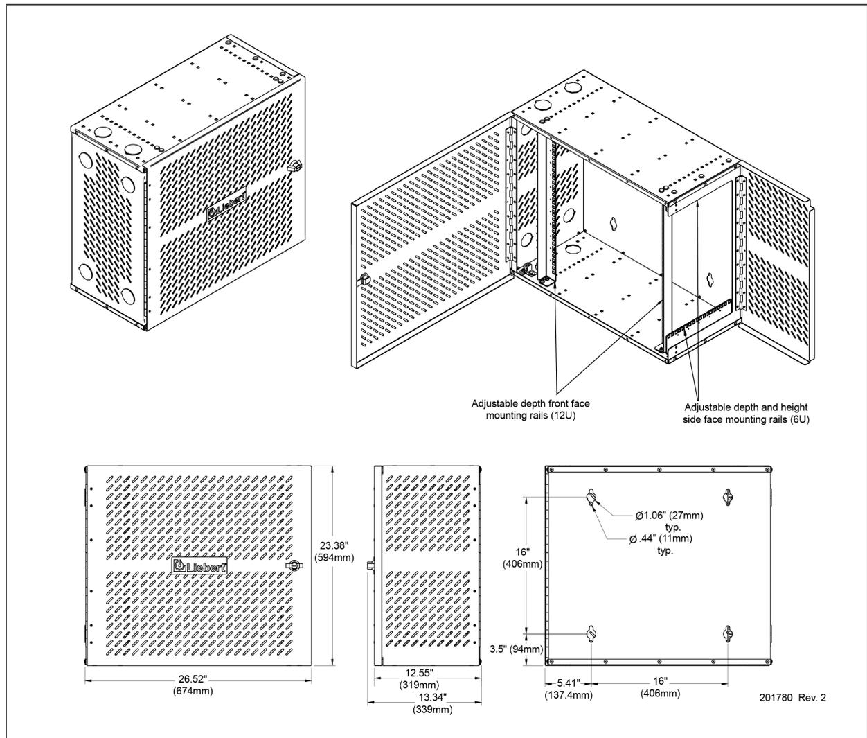
Figure 9.2 Liebert® MCR 12U hinged body wall-mount dimensions and features
