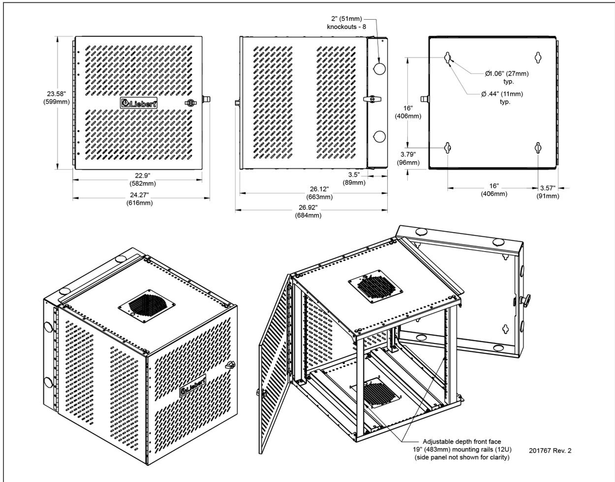
Figure 9.3 Liebert® MCR 22U Mini Computer Room with top-mount ECM dimensions and features
