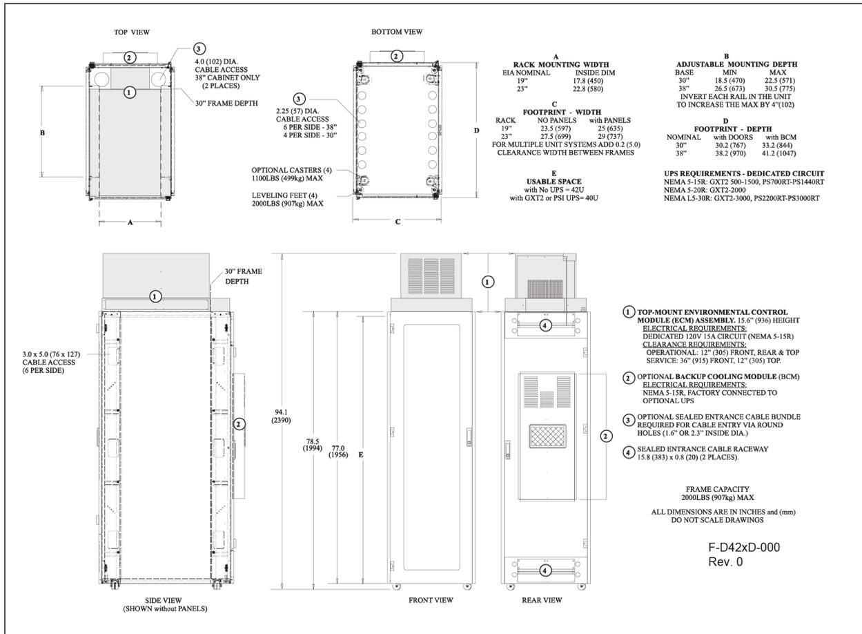
Figure 9.7 Liebert® MCR 46U Mini Computer Room with top-mount ECM dimensions and features
