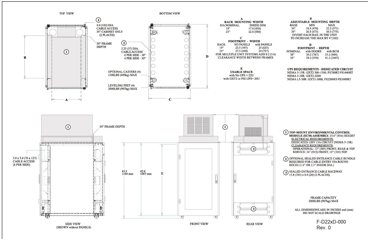
Figure 9.5 Liebert® MCR 42U Mini Computer Room with top-mount ECM dimensions and features
