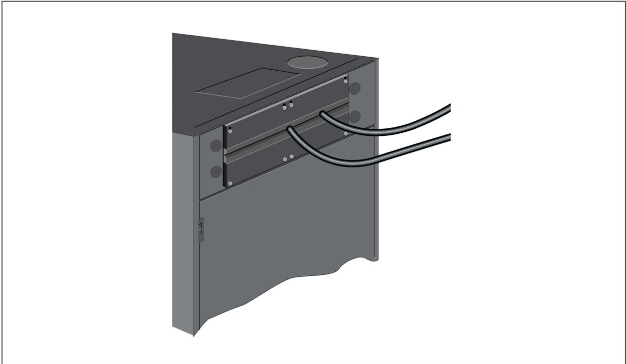
Optional sealed entrance cable bundles (cone-shaped seals and clamps) permit use of the round openings on the top and/or the bottom of the sealed Liebert® MCR for cable entry.
