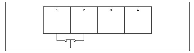
• To operate connected to a normally-open (NO) REPO connection, the jumper and the NO switch must be installed as shown in the figure.
