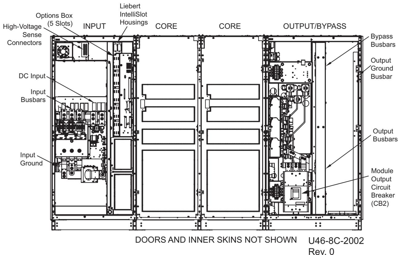
**Figure 4 Main component locations—1000kVA, 1100kVA, and 1200kVA (typical)**
