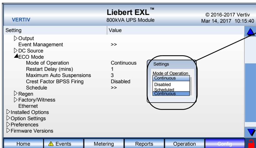
Select the type of Eco Mode operation to enable; Continuous operation is selected
