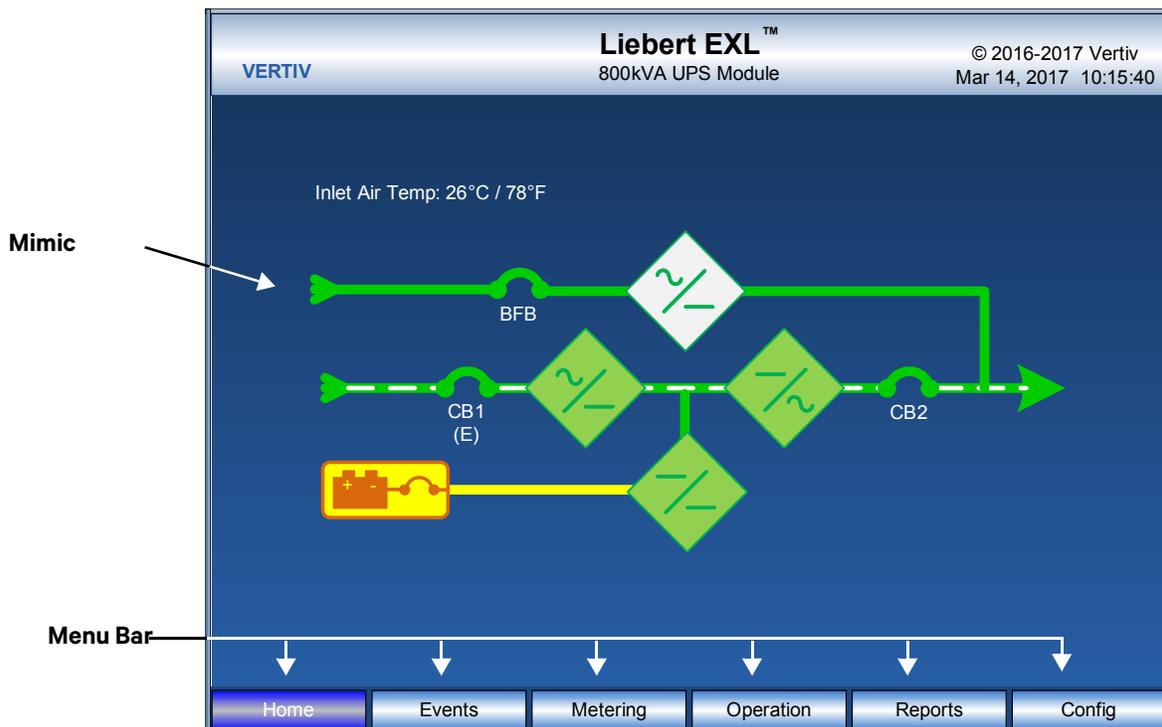
**Bypass Input**—The bypass circuit breaker (BFB) status is shown as Open or Closed.
