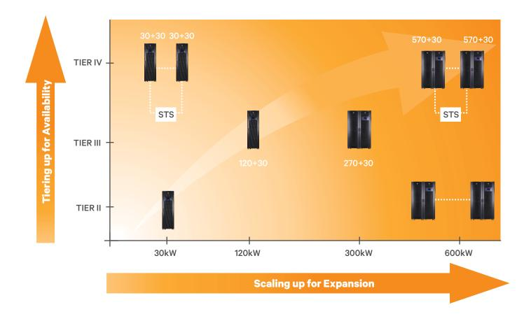
The Liebert® APM<sup>™</sup> system can be utilized with either single or dual power inputs. The dual power features allows you to take advantage of a secondary power source. In addition, up to 4 racks can be paralleled to achieve increased redundancy for more power and 2 sets of racks can be deployed in a Dual Bus architecture.
