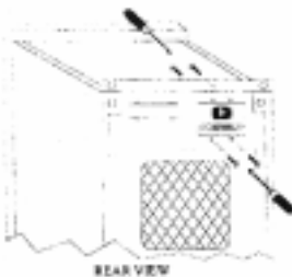
Figure 7 Installing New Option Plate
