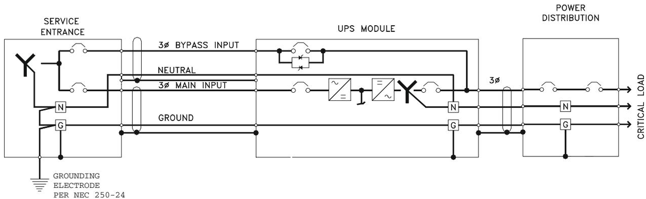
This arrangement may be used for systems with 208 VAC input and output. However, it does not provide any isolation or common-mode noise attenuation for sensitive loads. For this reason, this configuration is not a preferred installation method.
