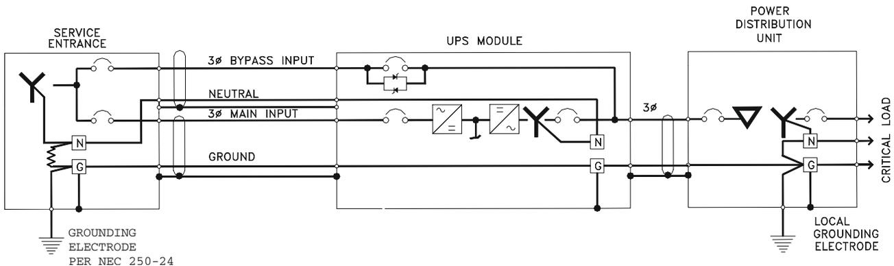
These configurations have the same restrictions as explained in **6.2 - Alternate Grounding Configuration, Wye-Connected Service**, except for the wye input. The UPS input and bypass must be fed from the same source. The load must be strictly 3-wire. And the GFI time delay should be set to at least 0.2 seconds to prevent tripping during transfer or retransfer operations.
