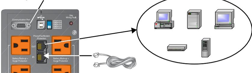
6. Press and release the ON/OFF/Alarm Silence button to turn on the UPS. The UPS will beep and the Utility Indicator will illuminate (green).
