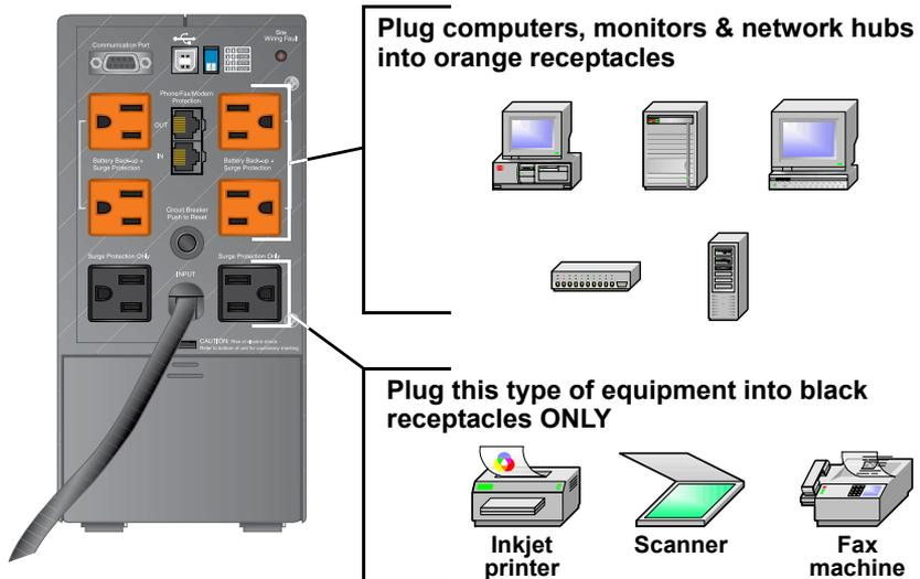
3. Plug the PowerSure PSA's attached 6-ft. (1.8m) power cord into an AC outlet. Check that the Site Wiring Fault Indicator on the rear is not illuminated. If it is lit, refer to the **Troubleshooting** section.
