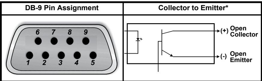
\* Maximum voltage and current on Pins 1, 7, 8, and 9 is 55VDC; 10.0 mA.
