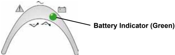
When a low battery condition occurs, the Battery Indicator changes to flashing amber and the alarm sounds every half-second. Low battery warning is defaulted to two (2) minutes but can be configured via MultiLink. For more information, refer to **Troubleshooting** section.
