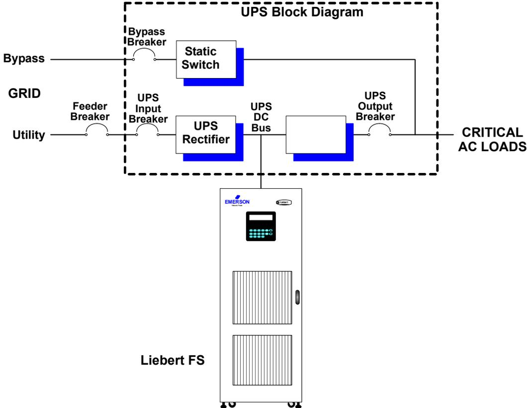
Several Liebert FS units can be put in parallel to achieve higher power output and higher ride-through duration (see **Figure 7**). One or more Liebert FS units may also be connected in parallel with a UPS battery plant (valve-regulated or wet cells) to provide an overall incremental reliability and life improvement for the DC battery plant. In this situation, the Liebert FS unit would be connected in parallel with the battery plant (through its own disconnect device) to the UPS DC Bus.
