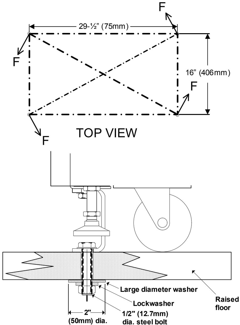
NOTE: Combination of floor material of given thickness , plus properties of large diameter washer and fastener , should result in lateral load capability to withstand shear due to load  $F = 1500 \text{ lb}$  (680kg), parallel to floor .
