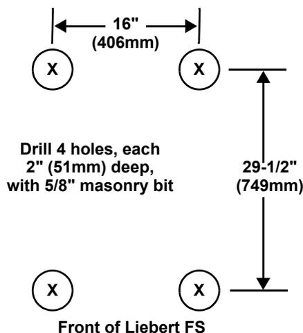
5. Drill 2" (51mm) deep holes in prepared surface using the drill bit included in the kit per bolt pattern described in **Figure 149 - Floor mounting template**. The setter rod should be used as a depth gauge to ensure proper depth. The setter rod is marked with two circles indicating the maximum and minimum hole depth allowed (see **Figure 18**).
