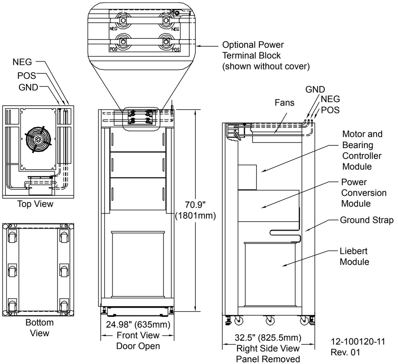
Figure 134 Liebert FS cabinet mechanical installation
