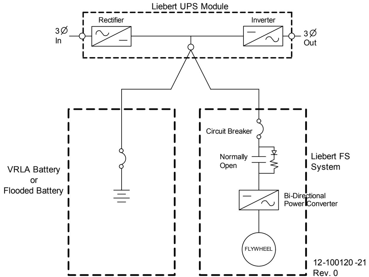
Figure 143 One-line diagram, single Liebert FS and battery with factory-integrated circuit breaker supplying Liebert UPS—UPS battery point of common connection
