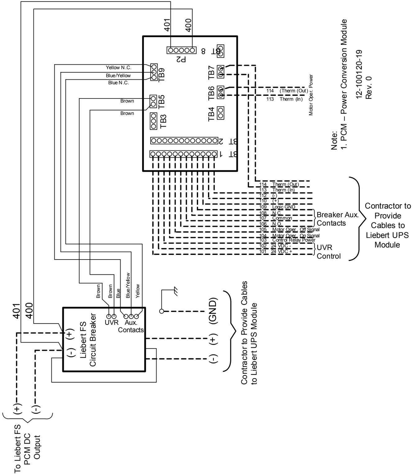
Figure 141 Two-eight paralleled Liebert FS units with factory-integrated circuit breaker in parallel with a Liebert UPS
