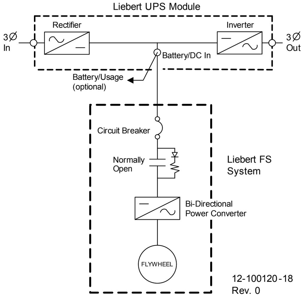
Figure 140 Control wiring diagram—Liebert FS - optional electrically operated circuit breaker Liebert Npower units
