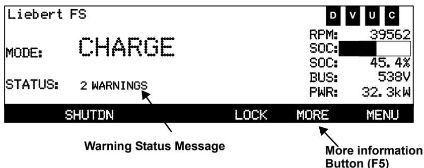
The Warning condition is indicated by the System Status field displaying “WARNING” in the Control Panel window (see **Figure 93**). If one Warning is present, the Warning Label (see **Table 15.**) will be displayed.
