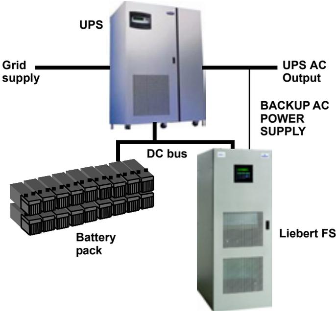
Figure 157 Multiple Liebert FS+DC units operating with a UPS in conjunction with batteries
