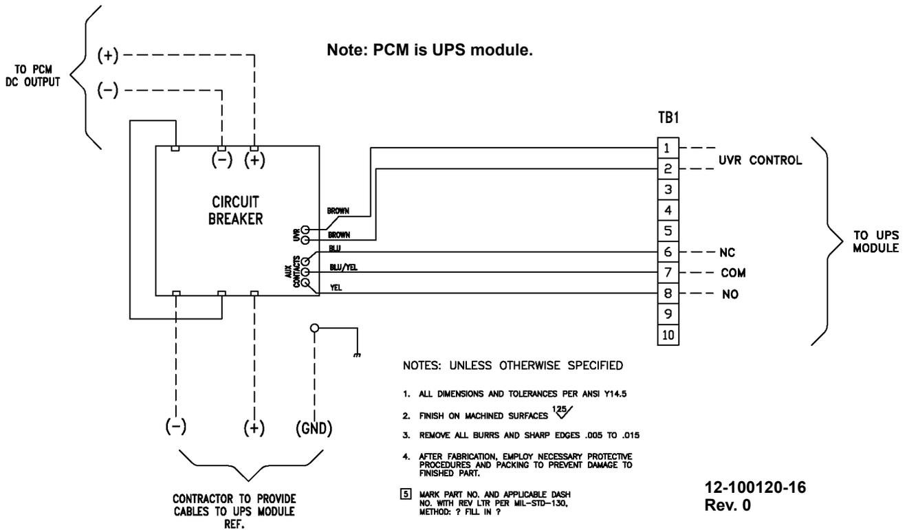
Figure 124 48 UVR, circuit breaker to terminal block wiring
