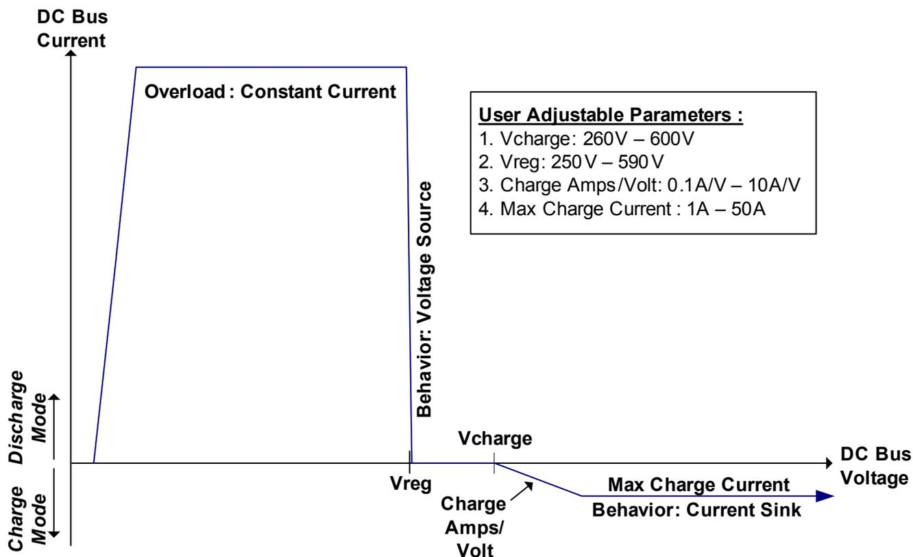
The V-I (Voltage and Inductance) curve (see **Figure 44**) shows the performance characteristics and modes of operation of the Liebert FS system based on the seven user-configurable system parameters.
