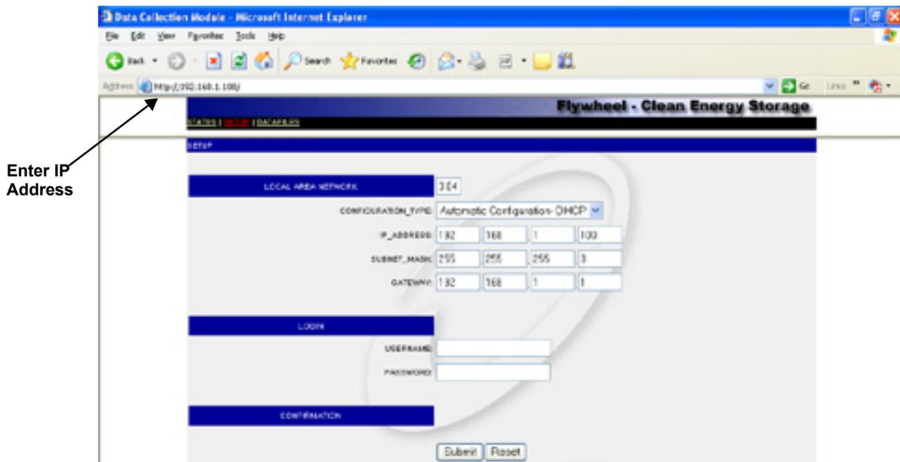
The DCM software has a screen menu bar along the top of the page. Three screens may be accessed: STATUS, SETUP and DATAFILES. The screens allow for setup of the DCM and different ways to browse the data recorded by the DCM.
