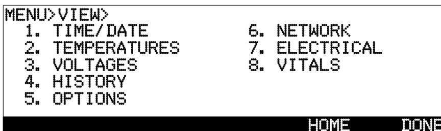
Selecting History will provide a history of Warnings and Faults as introduced in Section 5, Operations, of this manual. Other information that can be useful in troubleshooting are the Temperatures, Voltages, Options, Electrical and Vitals screens.
