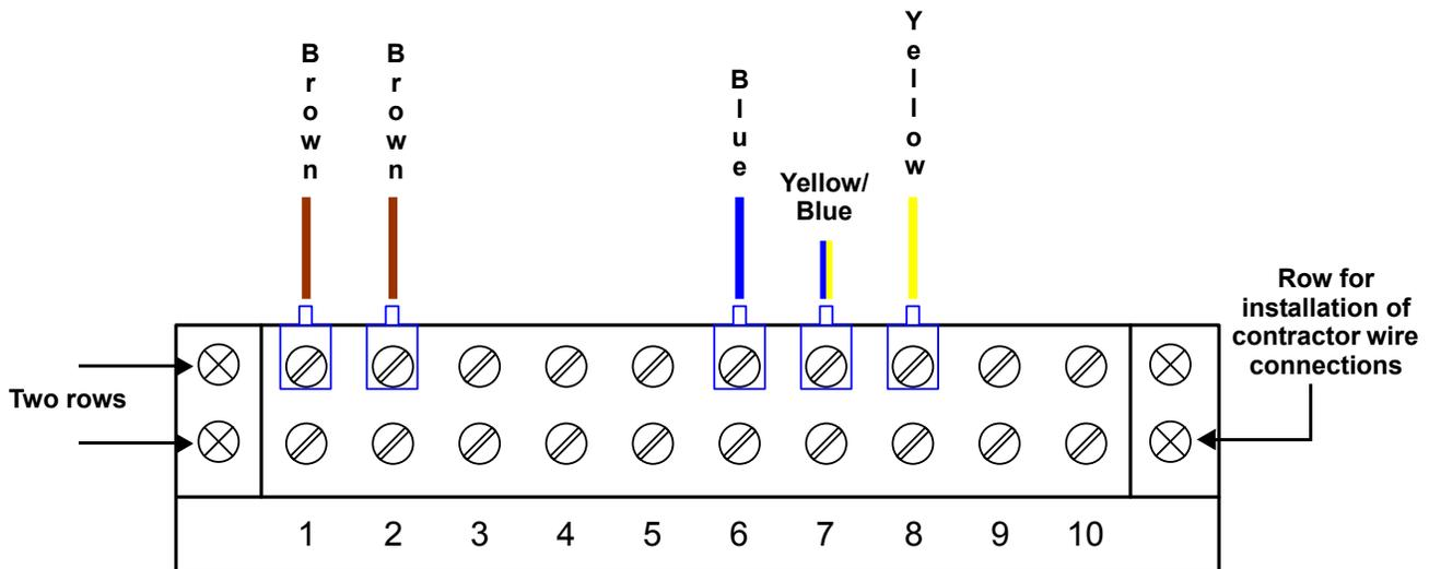
The recommended gauge for status/control connection wires is 16 AWG - 600VDC (1.3mm<sup>2</sup> wire section). Status/Control wires must be sized and installed in compliance with all applicable local, regional and national regulations (e.g., National Electric Code for USA).
