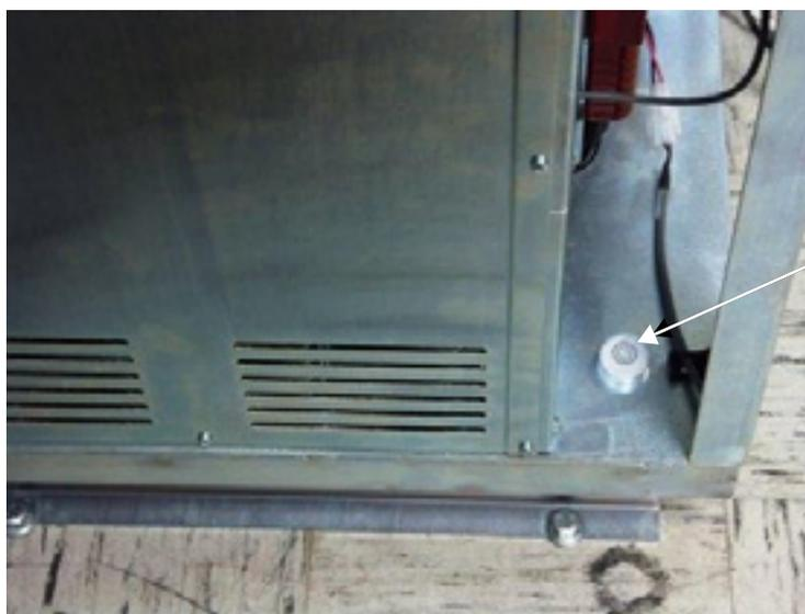
13. Once the cabinet is level, firmly tighten the front bolts to drop-in anchors as shown in **Figure 134**. The front bolts must be tightened to 40 foot-pounds (54 N-m) of torque.
