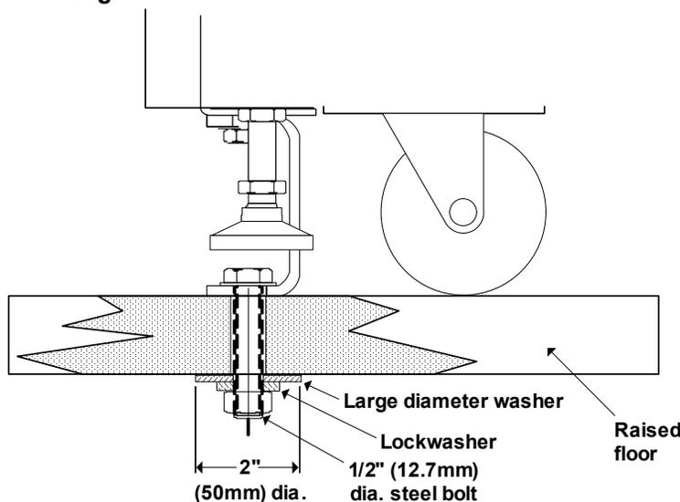
6. Attach a large diameter washer, a lock washer and a nut to each hex flange bolts as described in **Figure 25** and **Figure 155**.
