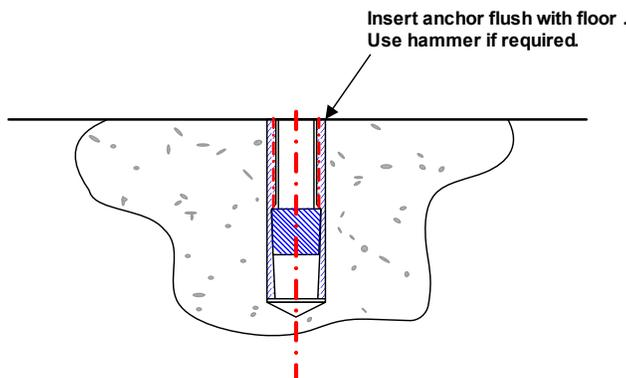
7. Tap anchors into drilled holes using hammer or mallet. When top of anchor is flush with mounting surface, use setter rod to expand and secure.
