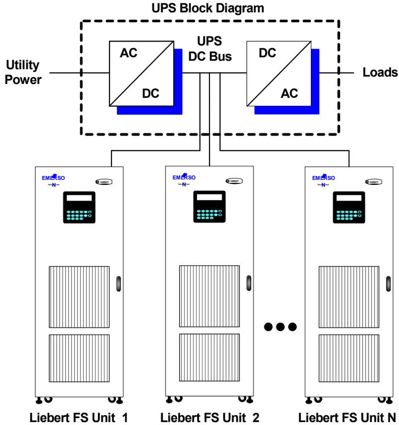
Figure 3 Liebert FS unit(s) integrated into UPS system for ride-through to backup generator
