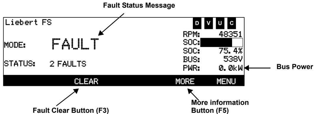
While in Fault condition, normal operation of the unit is suspended, the operation of the Power Conversion Module is paused, and the unit transitions into FAULT Mode, where it waits for one of the following to occur:
