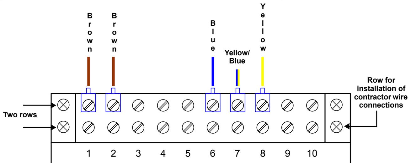
The recommended gauge for Status/Control connection wires is 16 AWG - 600VDC (1.3mm<sup>2</sup> wire section). Wire size and installation must comply with all applicable local, regional and national regulations (e.g., National Electric Code for USA).
