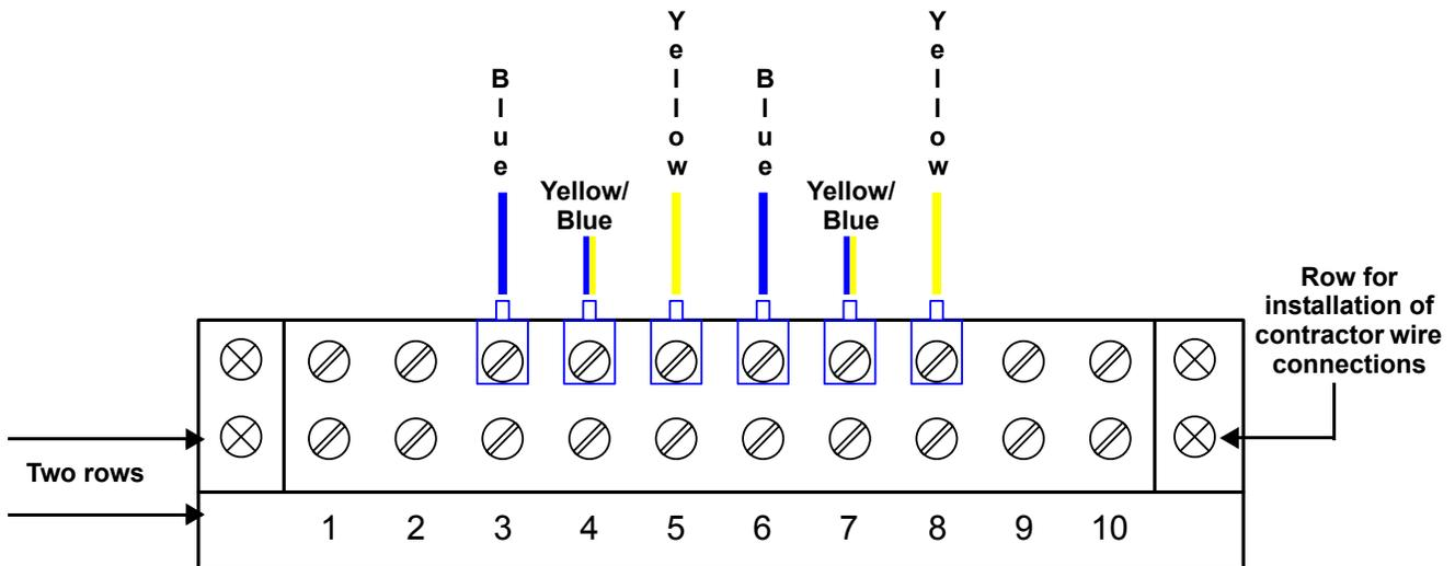
The recommended gauge for Status/Control Connection wires is 16 AWG – 600 VDC (approximate metric equivalent: 1.3 mm<sup>2</sup> wire section). All wiring must comply with all applicable local, regional, national regulations.
