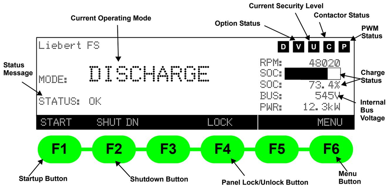
Figure 56 Fault screen functions
