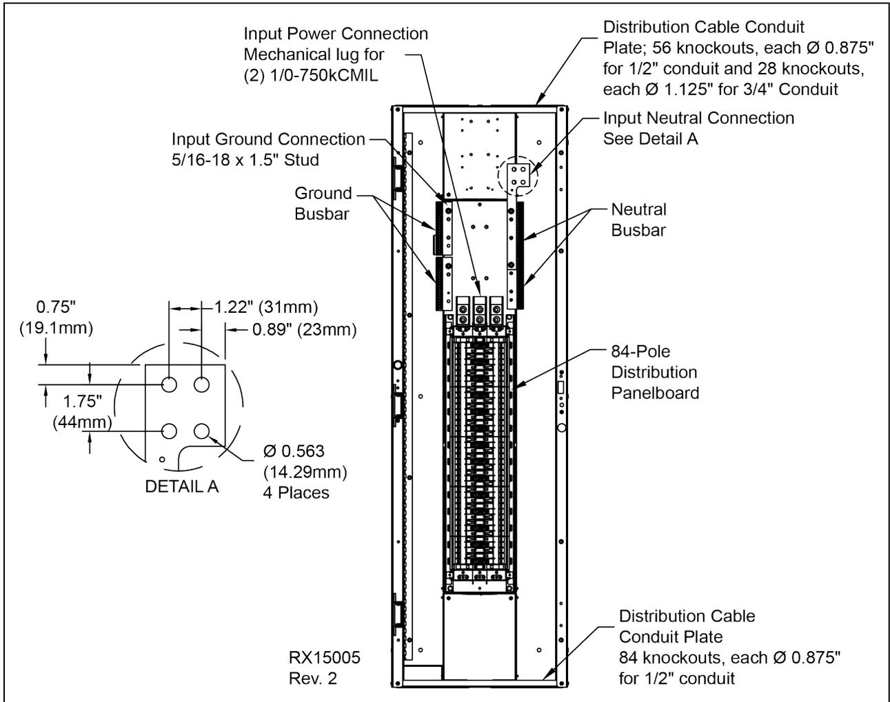
Figure 2.6 Electrical field connections for units with Vertiv™ Liebert® LDMF monitoring
