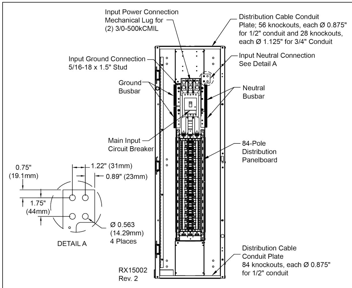
Figure 2.5 Input electrical field connection location for units without main panelboard breaker
