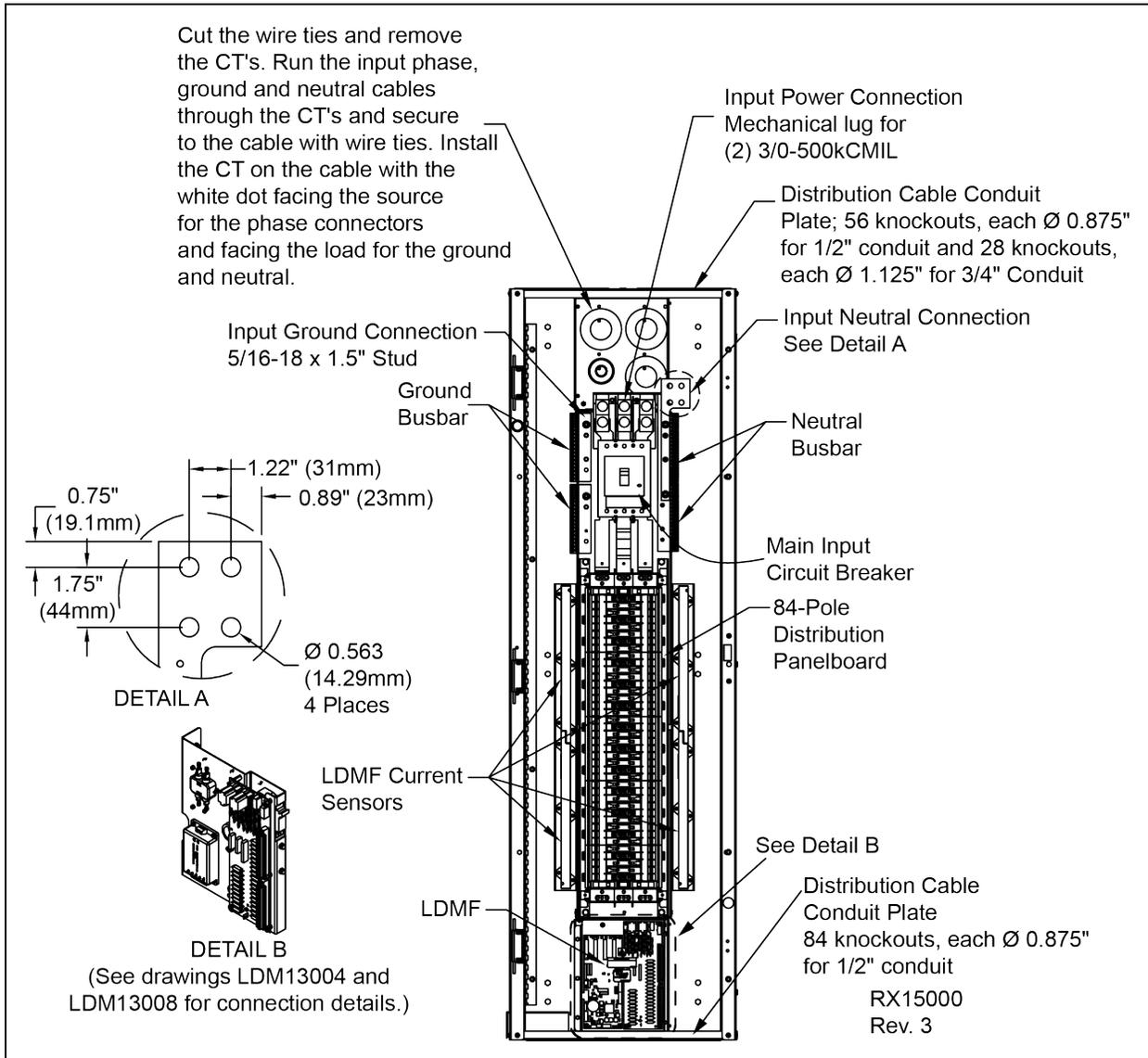
Figure 2.7 Electrical field connection for units with Vertiv™ Liebert® Current Plus Monitoring
