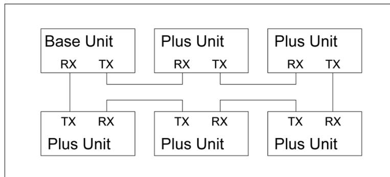
**Figure 51. Base to Plus Unit Connection**
