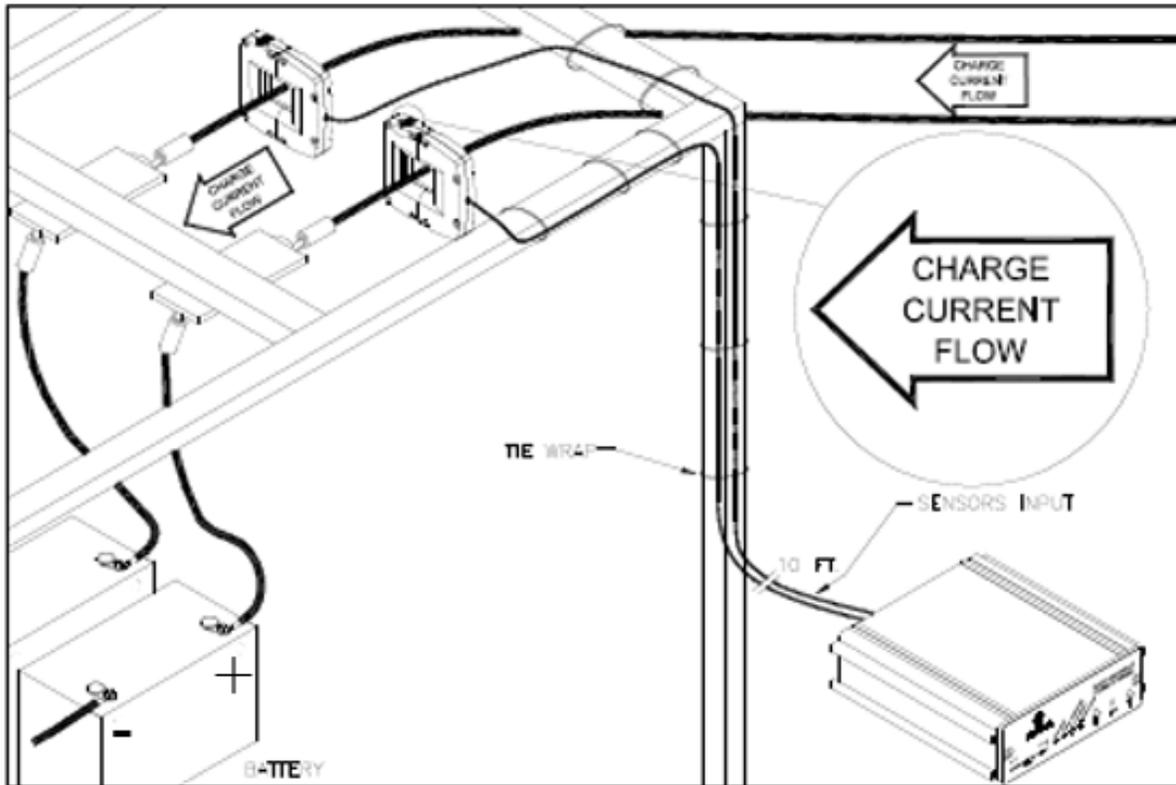
**Figure 47. From Multitel's FCCP Manual–Routing The Cable**
