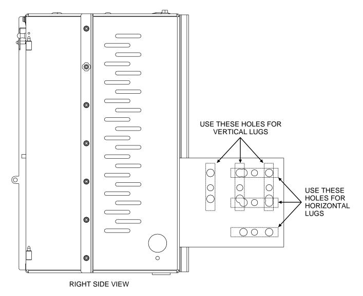
**Figure 4B:** Input and Output Connections with Optional Busbar Rear Extension Kit Installed (Input Busbar Shown; Output Busbar Similar.)
