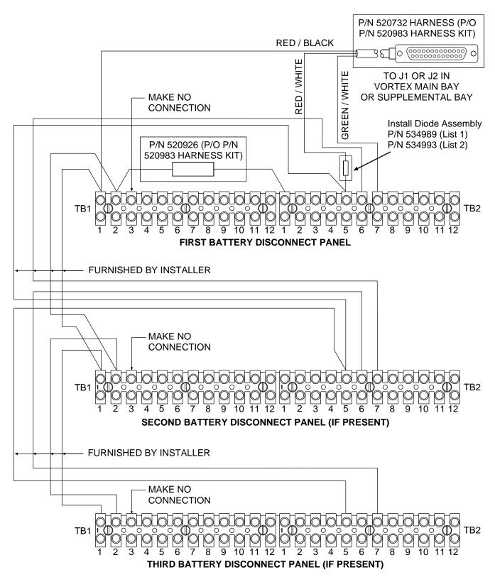
*Figure 8A:* Shunt POD Signal Interconnection with a Spec. No 581125000, 582125000 or 582126000 Main Bay or Supplemental Bay
