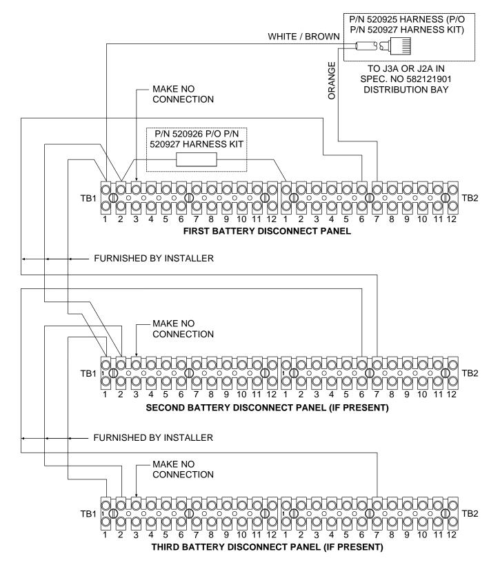
Figure 8C: Shunt POD Signal Interconnection with a Spec. No 582121901 Distribution Bay
