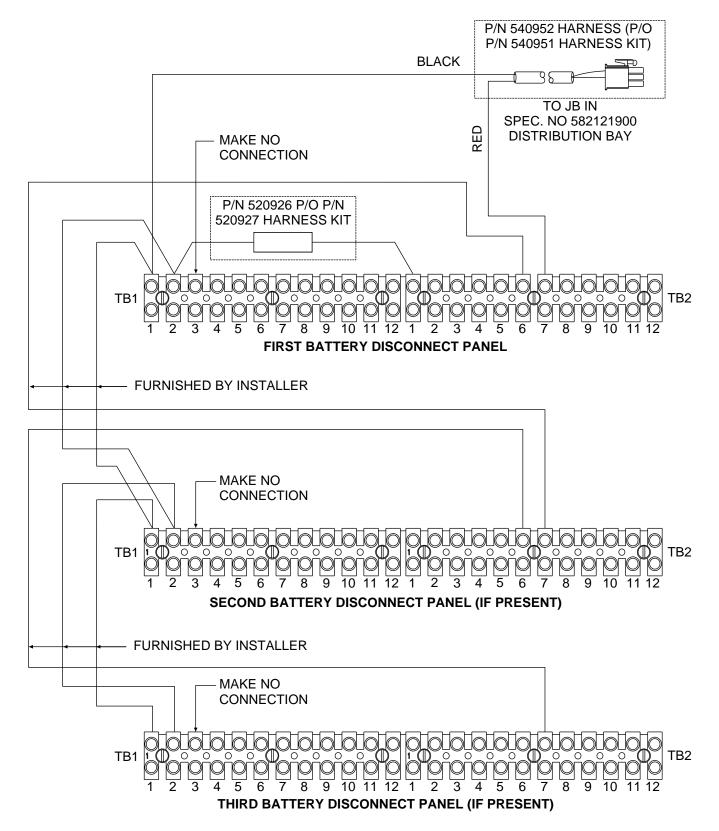
*Figure 8B:* Shunt POD Signal Interconnection with a Spec. No 582121900 Distribution Bay
