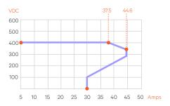
Figure 2: Output Voltage vs. Output Current at Maximum Output Power 15000 W
