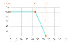
Figure 3: Output Power vs. Temperature at Uin > 340 VAC, Vo > 336 VDC
