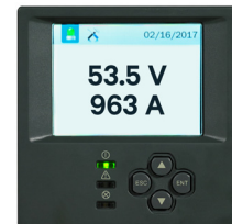
Figure 1: Home page of the DMU showing total voltage and current.
