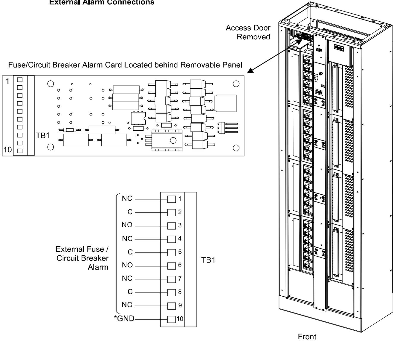
\* May be strapped to terminal 2, 5, or 8 to provide switched ground, if required.
