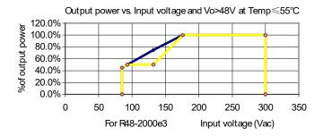
**NOTE!** Blue Line: Linear derating from 85V AC to 176V AC. **Yellow Line:** Linear derating from 2000 watts at 176V AC to 1000 watts at 132V AC. Constant 1000 watts from 132V AC to 93V AC.
