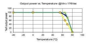
NOTE! Green Line: at 200Vac < Vin < 250Vac and 50Vdc < Vout < 56Vdc.</li>
