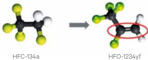
**Figure 5:** Hydro Fluorocarbon (R134a) and Hydro Fluoro Olefin (R1234yf)
