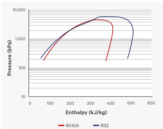
R32 density is lower than R410A, so it has a lower pressure drop with increasing efficiency and requires lower refrigerant charge. R32 works with high  $\Delta T$  on the heat exchanger, this means that for the same cooling capacity,
