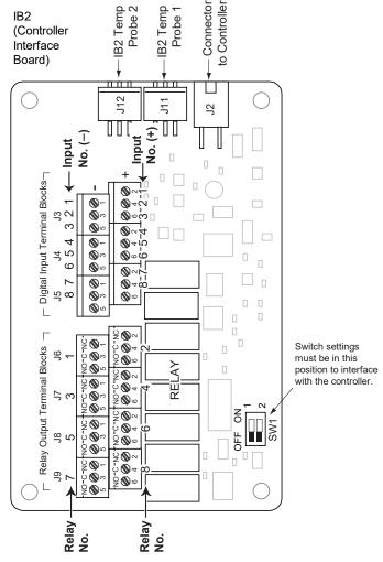
The controller relay assigned to "Critical Summary" alarm (relay 1 by default) will operate in the "Fail Safe Mode". "Fail Safe Mode" means Relay 1 is de-energized during an alarm condition, opening the contacts between the C and NO terminals, and closing the contacts between the C and NC terminals.
