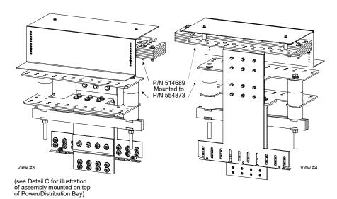
External Top-Mount Ground (Load Return) Busbar Assemblies (for use with External Top-Mount Battery Input Busbar Assembly P/N 554873)
