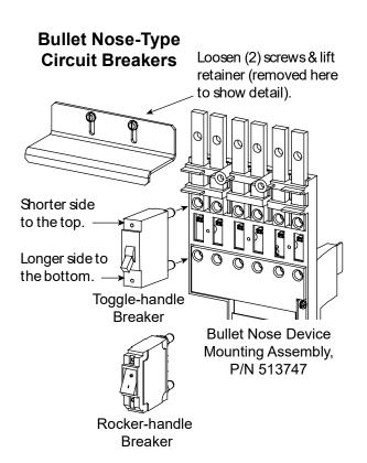
Note: Load leads are connected to the existing load busbars provided at the top of the bay. These busbars provide 1/4" studs on 5/8" centers and hardware for installation of customer provided two-hole lugs.
