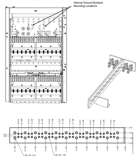
Internal Ground Busbar Assembly P/N 555214
