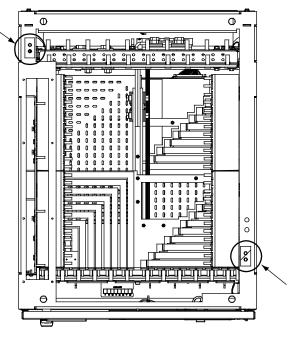
Top View Power/Distribution Bays (Power Only Bays Similar) Two holes with 1/4-20 captive nuts provided for installation of customer provided two-hole lug with 1/4" bolt clearance holes on 5/8" centers
