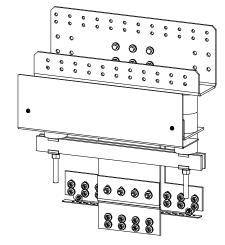
External Top-Mount Vertical Battery Input Busbar Assembly, P/N 554874
