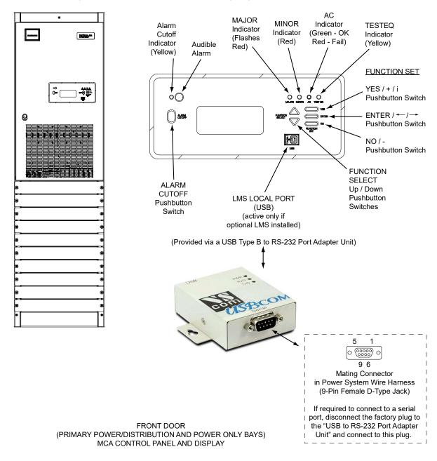
Navigating the MCA is an easy process. You just have to remember a few key combinations (as shown in the following chart). The symbols that appear at the end of the fourth line of the display indicate which keypad buttons can be pressed at any given time.
