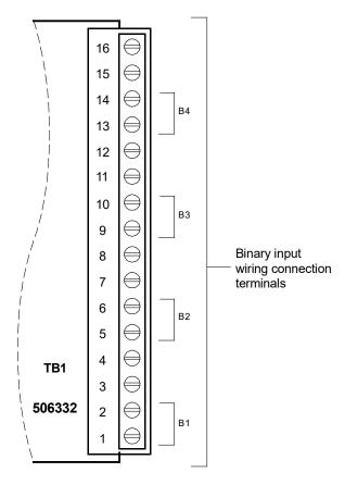
Note: Binary input designations B1 through B4 as shown are for the circuit card only. The actual binary channel number depends upon the quantity of binary circuit cards installed and the location of this binary circuit card in the system network.
