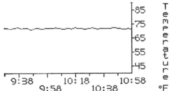
Histograms—historical depictions—of temperature or humidity can be displayed on the screen for analysis. This is especially helpful in tracking the environmental factors of an alarm.
