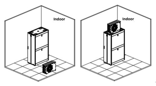
Figure 2-10 Standard Condensing Unit Without Air Deflector for Indoor Use
