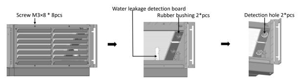
Figure 7-4 Detection Holes in VRC202 (Front)
