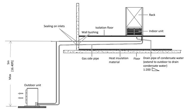
*Figure 3-12* shows the scenario where the condensing unit is installed lower than the indoor unit.
