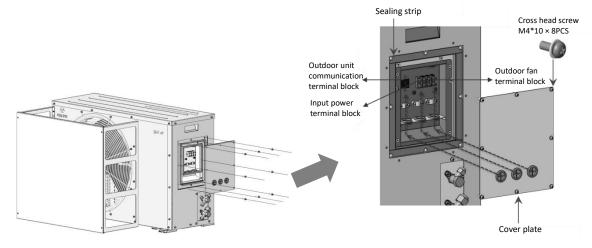
Input cabling connections of the condensing unit power terminal block are shown in *Figure 4-5*.
