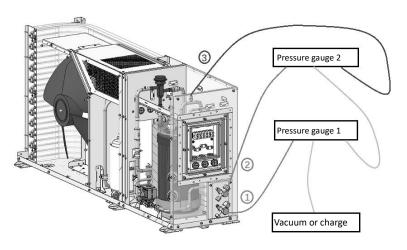
Figure 3-28 Vacuuming and Charging for Low Ambient Condensing Unit
