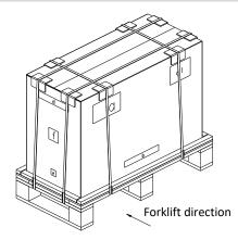
**Figure 2-5 Forklift Direction**
