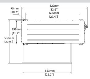
Figure 3-9 Standard Condensing Unit Top View
