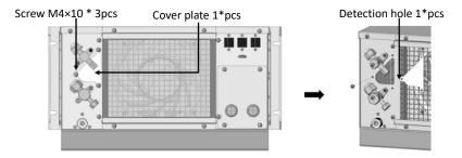
Figure 7-5 Detection Holes in VRC202 (Rear)
