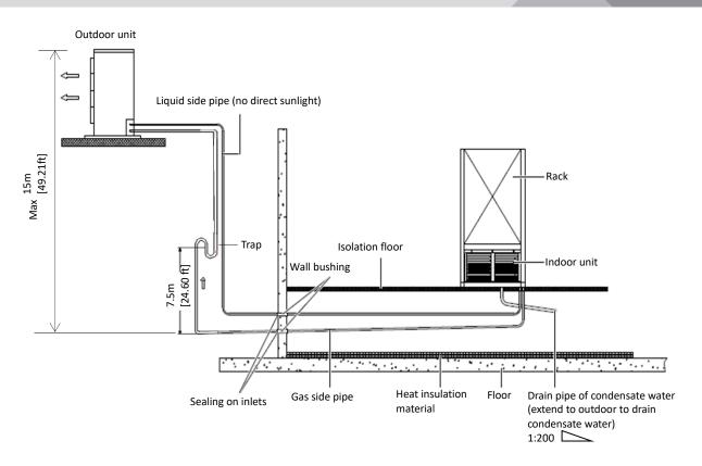
Figure 3-11 Condensing Unit Installed Higher Than the Indoor Unit
