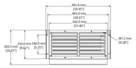
Figure 3-6 Front View of Indoor Unit
