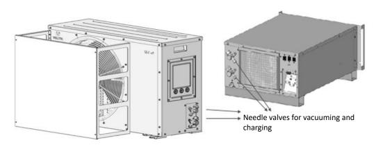
Figure 3-27 Charging the Refrigerant Gas
