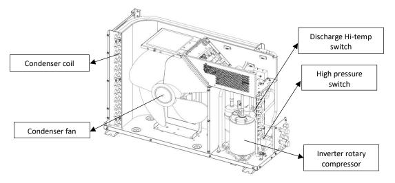
Figure 1-7 Standard Condensing Unit Internal Parts
