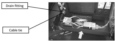
Figure 3-18 Installation of The Pump Kit
