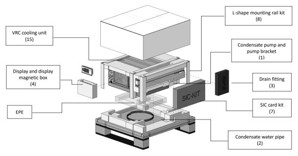
Figure 2-7 Unpacking Indoor Unit
