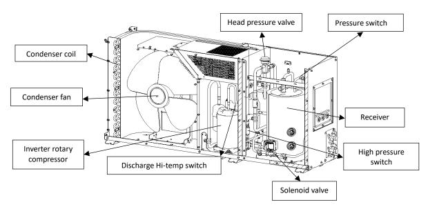
Figure 1-8 Low Ambient Condensing Unit Internal Parts
