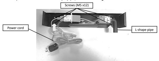
Figure 3-17 Internal Structure of Water Pump Bracket
