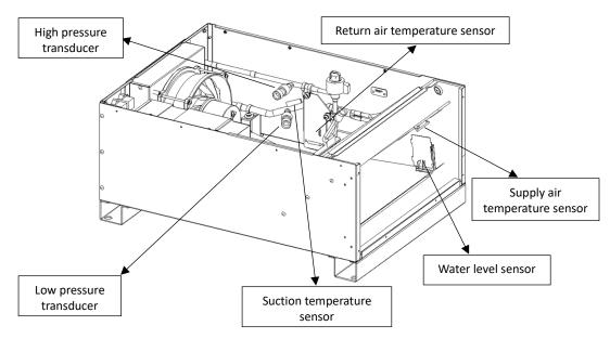
Figure 1-6 Indoor Unit Sensor Location
