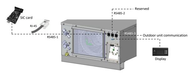
Figure 4-8 Communication and Monitoring Cable Connections in the Indoor Unit
