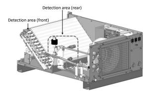
Figure 7-6 Detection Area in VRC202 (Rear)
