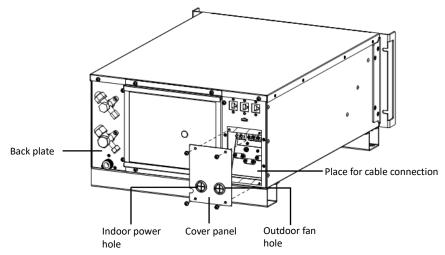
Figure 4-1 Cover Panel for Cabling Connections
