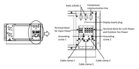
Figure 4-4 Input Cabling Connections – Indoor Power Terminal
