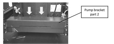
Figure 3-19 Installation of The Pump Bracket Part 2
