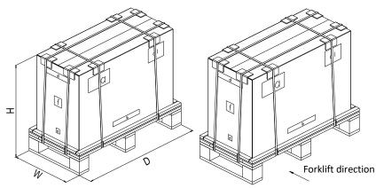
Figure 2-3 Package Dimensions – Condensing Unit
