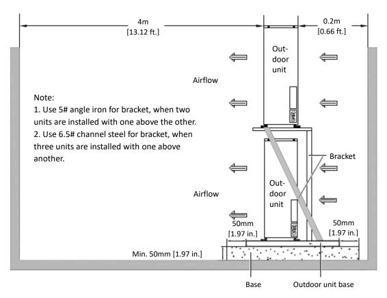
Figure 3-13 Installing Multiple Condensing Units with One Above the Other
