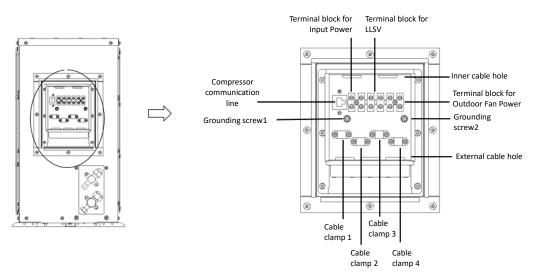
Figure 4-7 Low Ambient Condensing Unit Electric Connection Illustration
