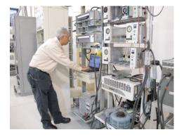
Firmware is updated and equipment is tested within a compatible system to ensure proper operation.
