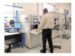
Specially designed ATEs (Automated Test Equipment) are used to calibrate and perform a full array of tests to verify that refurbished or upgraded equipment operates as originally designed.
