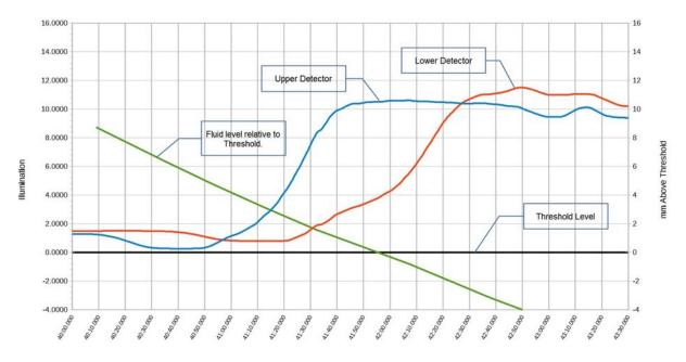
Figure 4. Graph of IR Receiver Output Samples for the Two Detectors as the Electrolyte Level Falls
