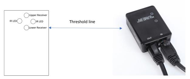
Figure 3. Optical Placement Diagram for the Infrared Level Detector
