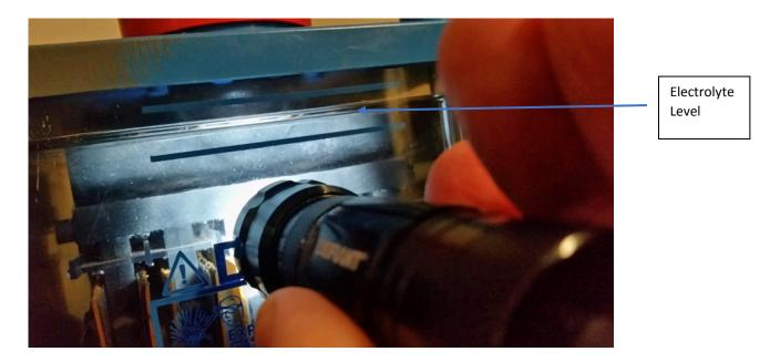
Figure 1. Light Below the Liquid Level
