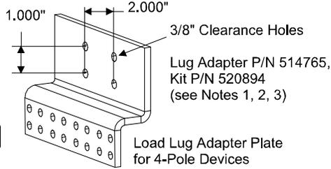
Load Lug Adapter Plate for 4-Pole Devices
