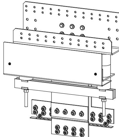
External Top-Mount Vertical Battery Input Busbar Assembly, P/N 554874
