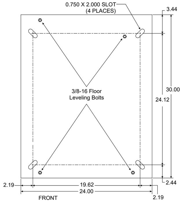
**Floor Hole Drilling Pattern Dimensions - Power/Distribution Bay and Power Only Bay (with AC Input Service Cabinet)**
