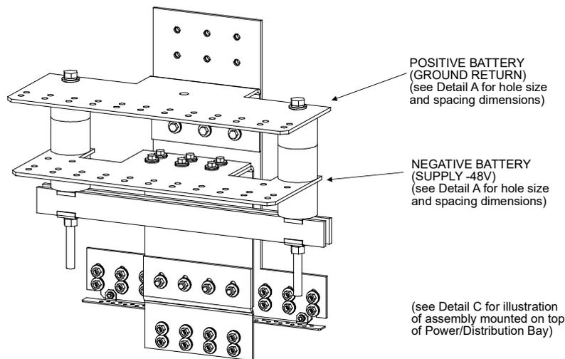
External Top-Mount Battery Input Busbar Assembly (P/N 554873)
