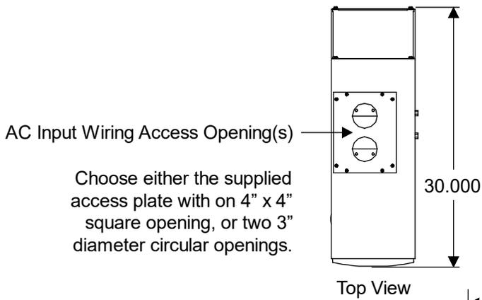
Choose either the supplied access plate with one 4" x 4" square opening, or two 3" diameter circular openings.
