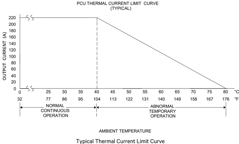
(D) High Temperature Inhibit: A thermal switch present in each rectifier continuously monitors the temperature of the power conversion circuit. If the temperature of the power conversion circuitry exceeds the design limits a circuit will inhibit the rectifier. Manual restart is then required.
