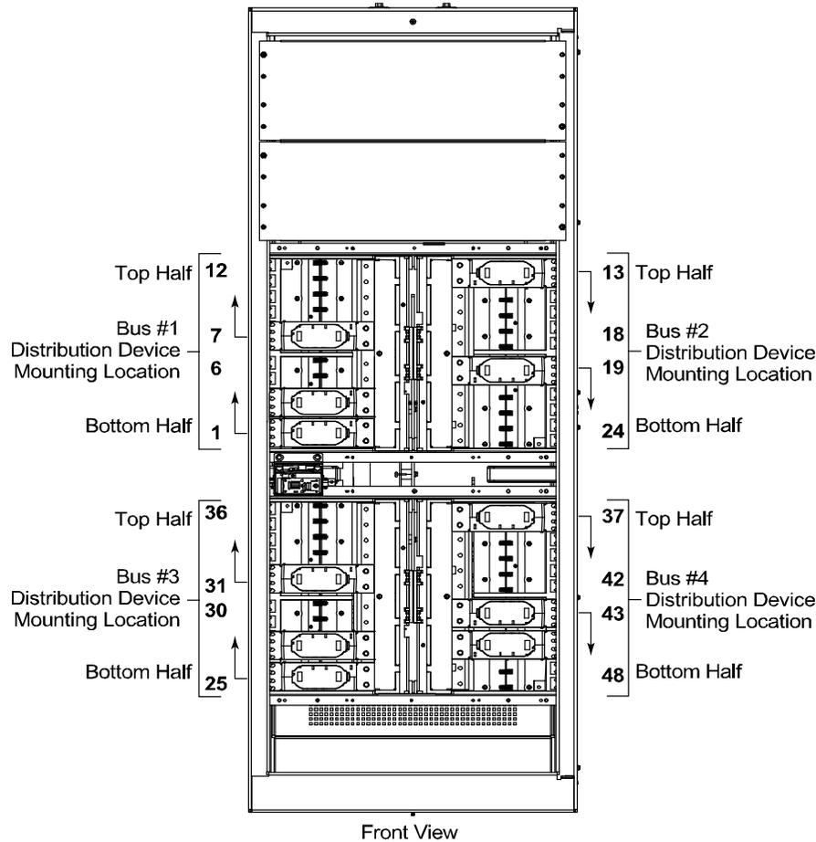
Note: On the left side, each half of each bus **MUST** be populated with distribution devices from bottom-to-top, without skipping any distribution device mounting positions within each half. (Arrows indicate starting position in each half.)
