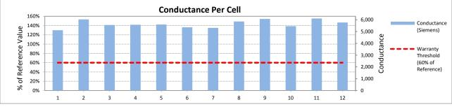
Figure 3. Ohmic Readings
