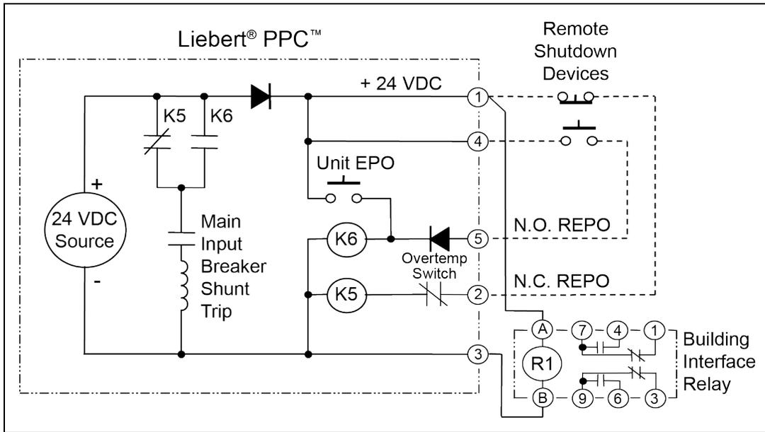
Figure 1.10 Typical Control Wiring for Power Monitoring
