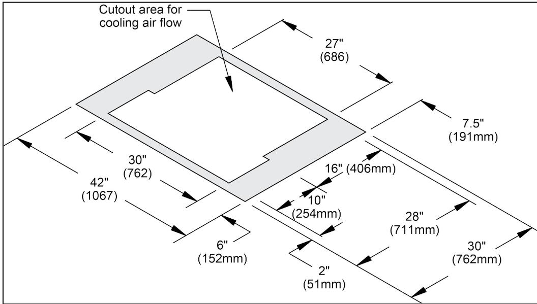
Figure 1.4 Footprint and Floor Cutout Dimensions for Transformer Section - 800kVA Units
