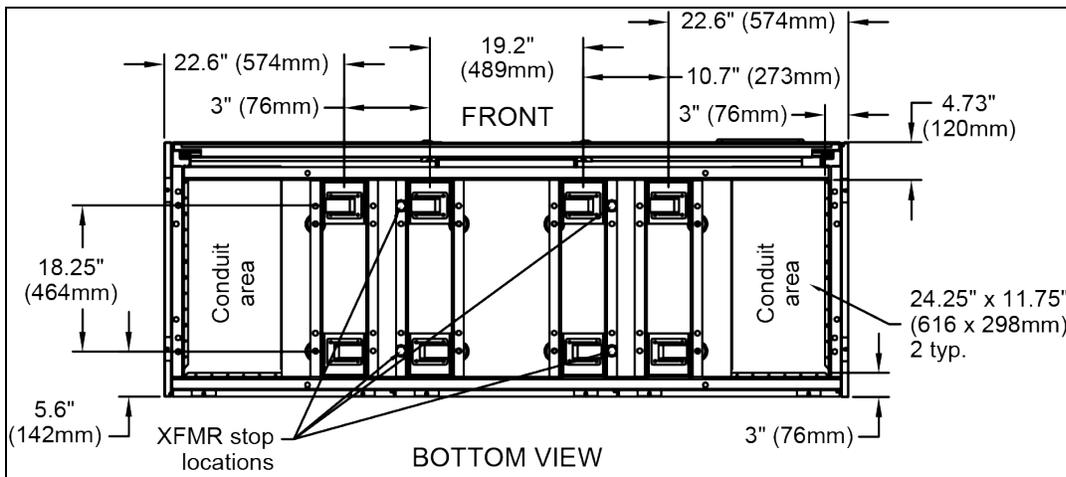
**Figure 1.5 Footprint and Floor Cutout Dimensions for Distribution Sections - 150-800kVA Units**
