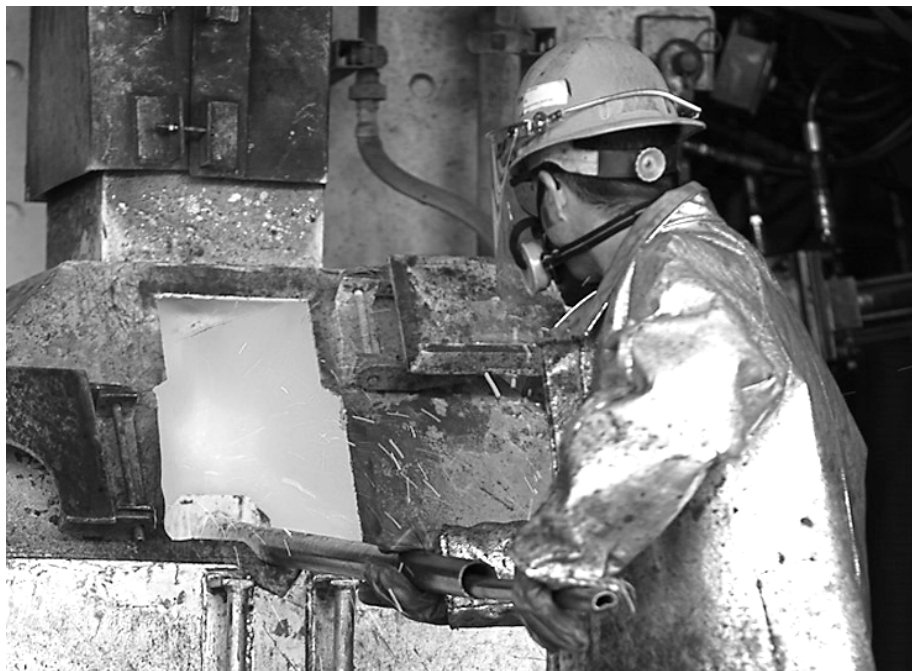
Figure 5. Tapping Slag from the cupola.
