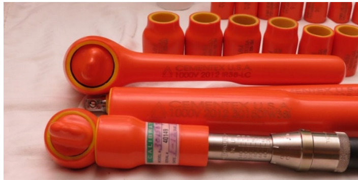
Figure 11. Insulated Torque Wrench with Removable Sleeve and Sockets.
