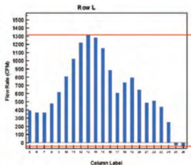
**Airflow analysis across one row of racks using floor mount precision air conditioners with 18-inch raised floor.**
