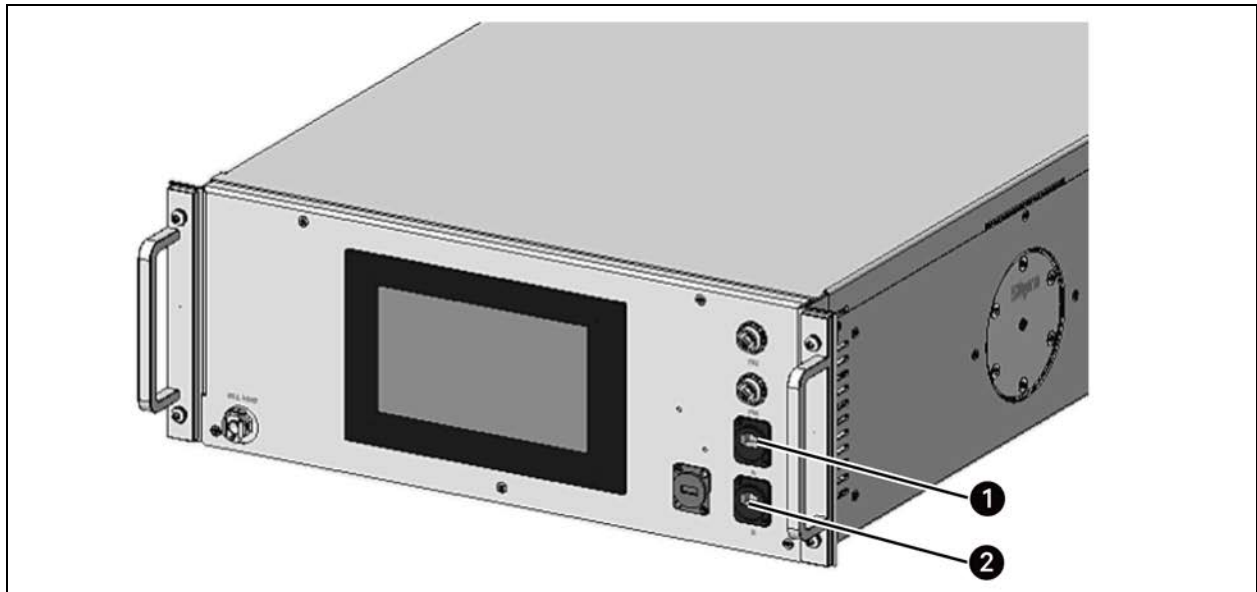
Figure 5.5 CoolChip CDU 121 Ethernet Connections
