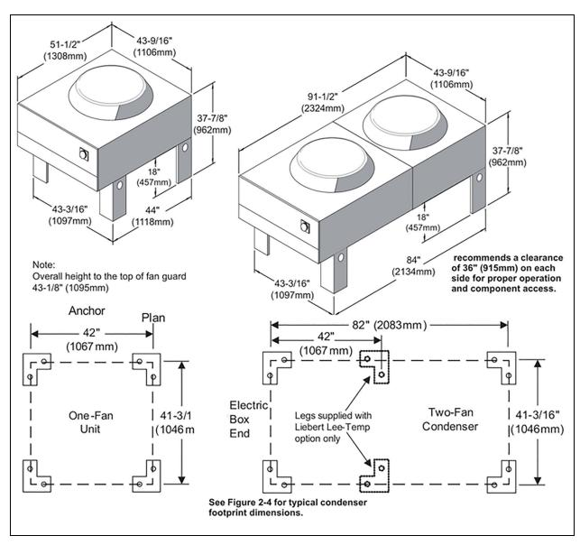
Figure 3.1 Condenser Planning Dimensional Data—1- and 2-Fan Units
