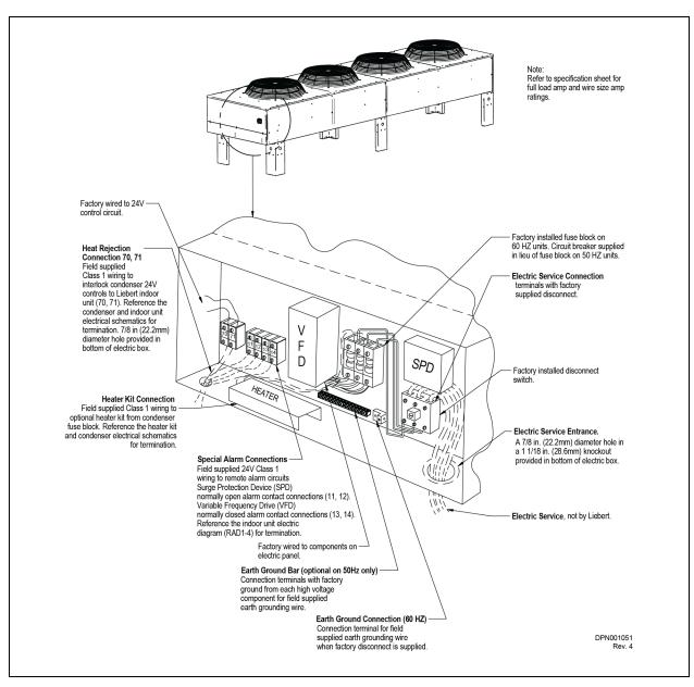
Figure 6.4 Electrical Field Connections for VFD Control Condensers
