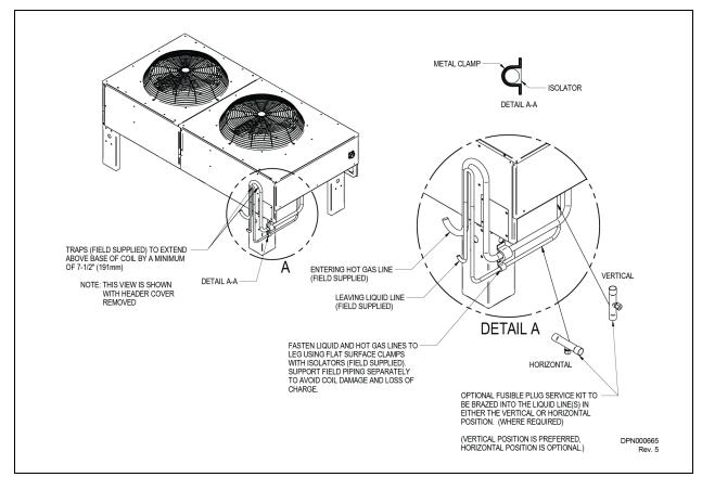
Figure 5.5 Single Circuit Piping, VFD and Fan Speed Control, 1-4 Fan Condensers
