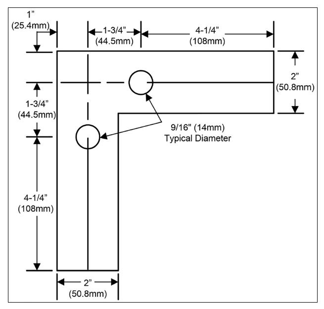
Figure 3.4 Typical Fin/Tube Condenser Footprint—Dimensions
