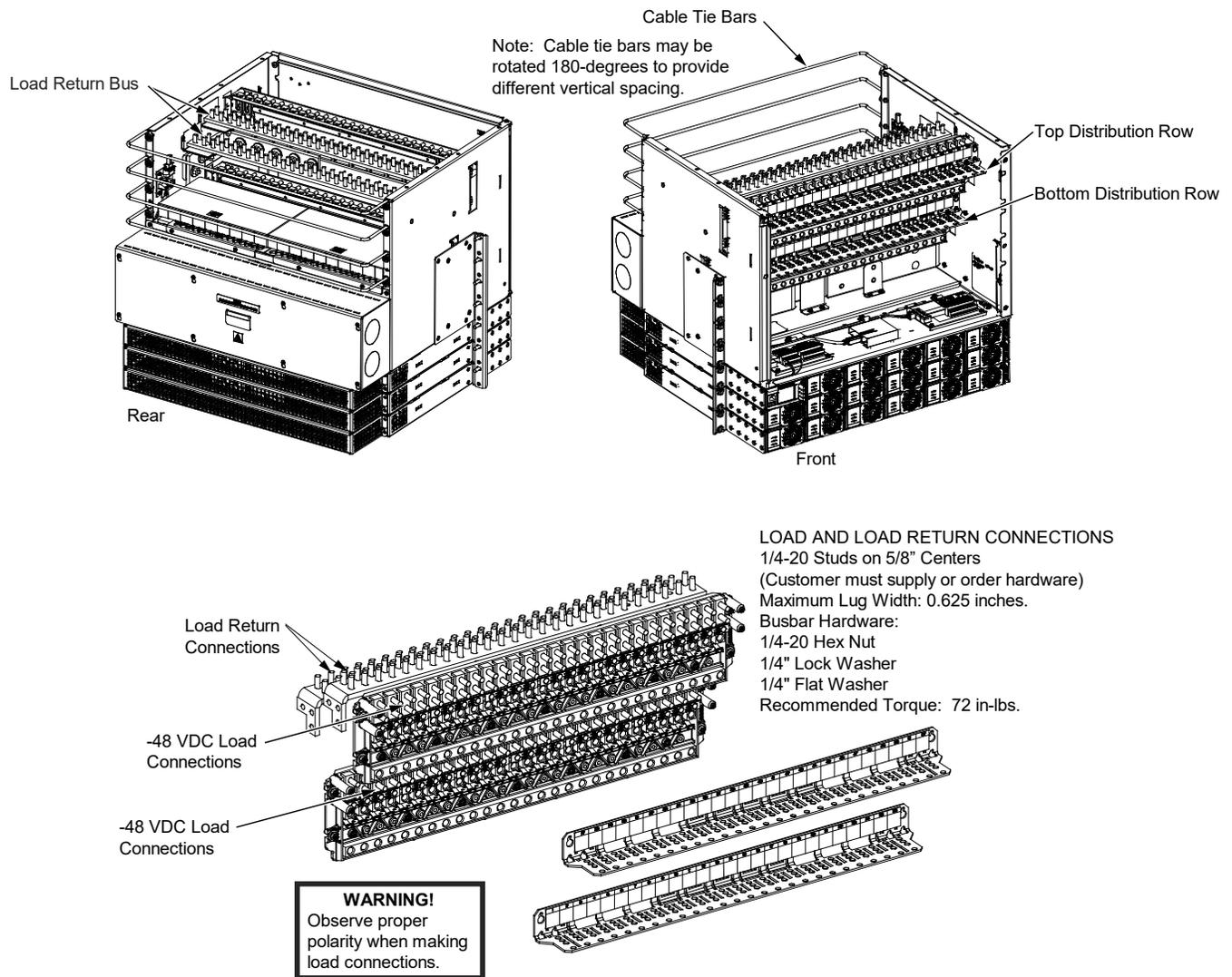
Note: 80 A circuit breakers can be used without a space provided the continuous current in each 80 A device does not exceed 51 A. A 100 A or greater circuit breaker SHALL HAVE an empty mounting position between it and any other overcurrent protective device.
