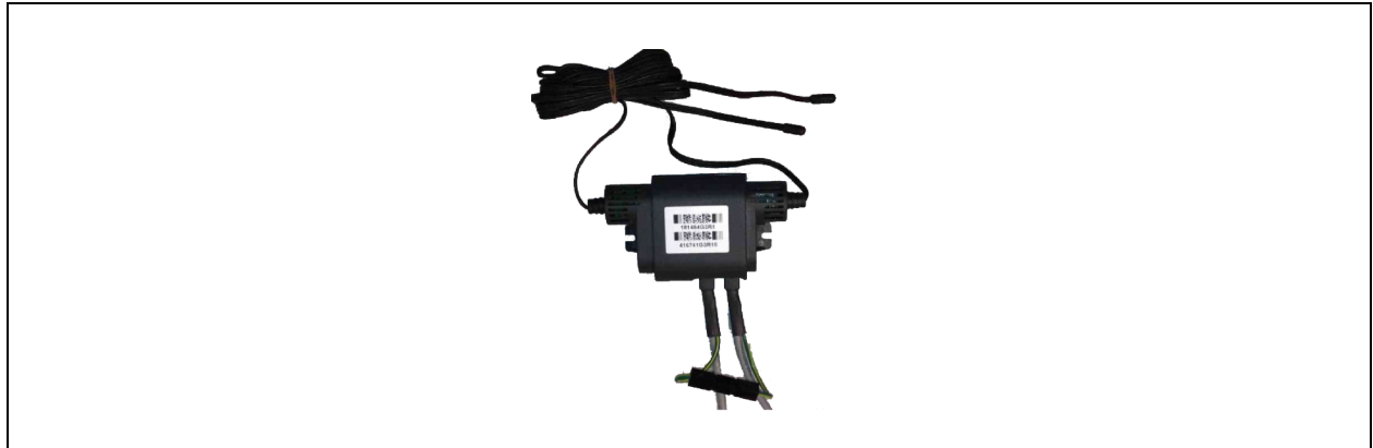
Figure 12.16 CANbus and Ground Connection on 2T Sensor
