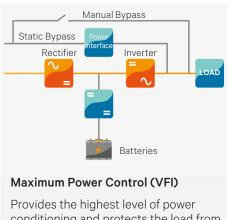
Provides the highest level of power conditioning and protects the load from all electrical network disturbances.
