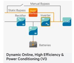
Compensates the load THDi, PF, main sags and swells, ensuring fast transfer output performance.
