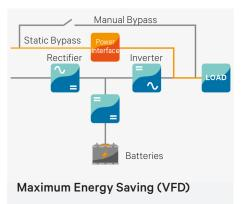
Detects when conditioning is not required and allows the energy flow to pass through the bypass line.
