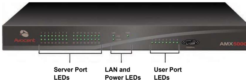
Figure 2.14: AMX Switch LEDs (AMX 5000 Switch Shown)
