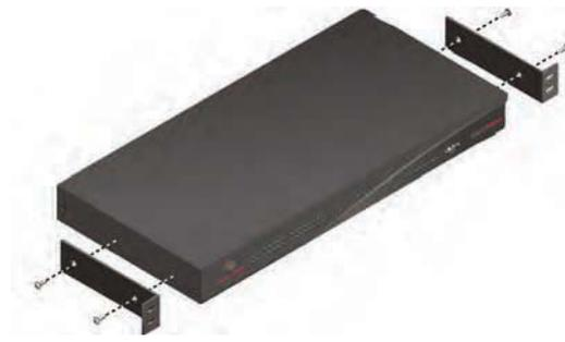
Figure 2.5: AMX Switch Rack Mounting Diagram
