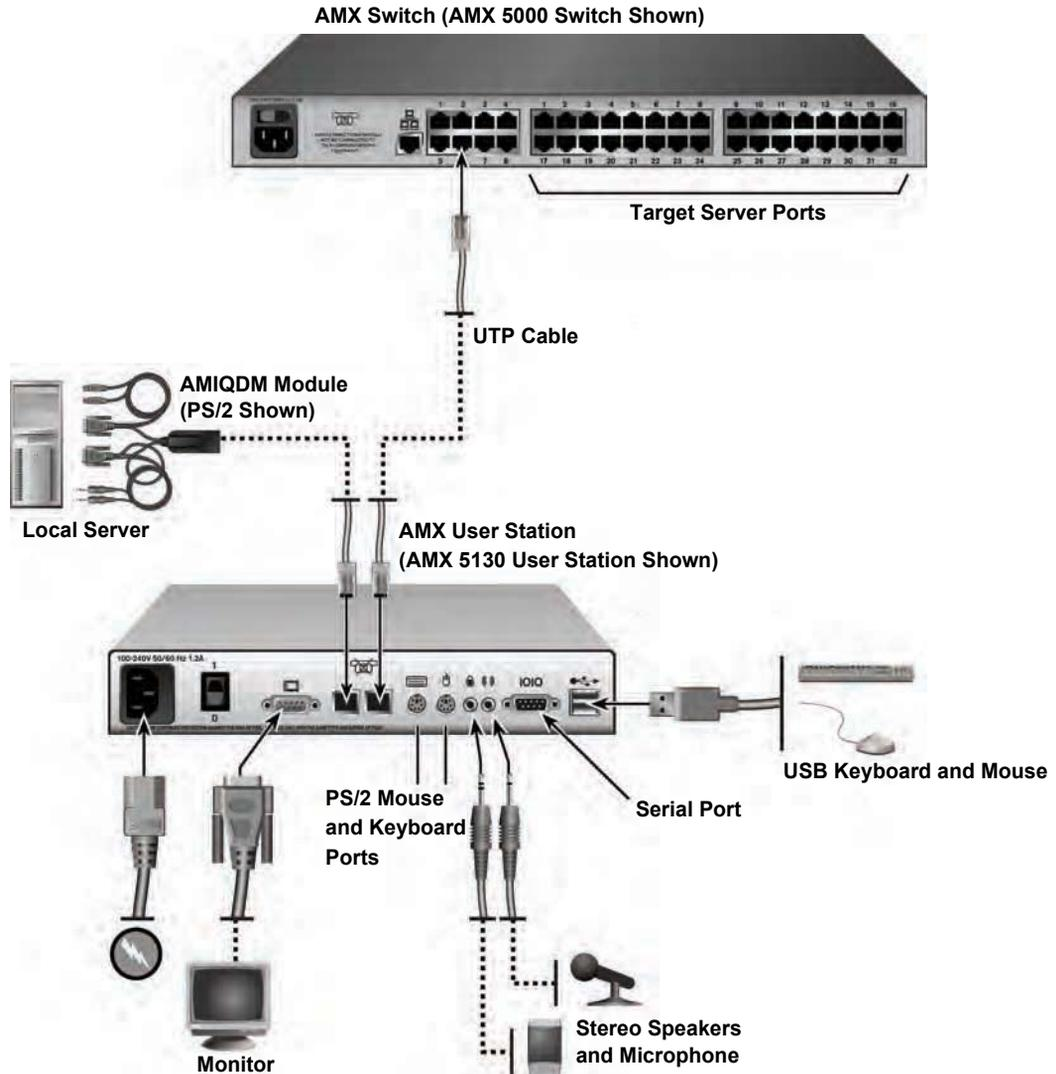
Figure 2.8: Connecting Users to an AMX Switch
