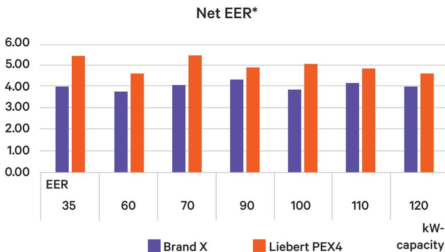
\* EER is calculated at return air condition of 33°C RH & condensing temp of 45°C
