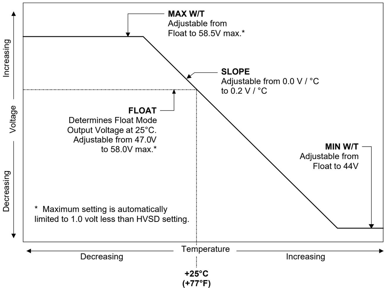
Typical Float Charge Thermal Characteristics
