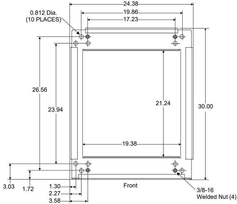
**Floor Hole Drilling Pattern Dimensions - Distribution Bays**
