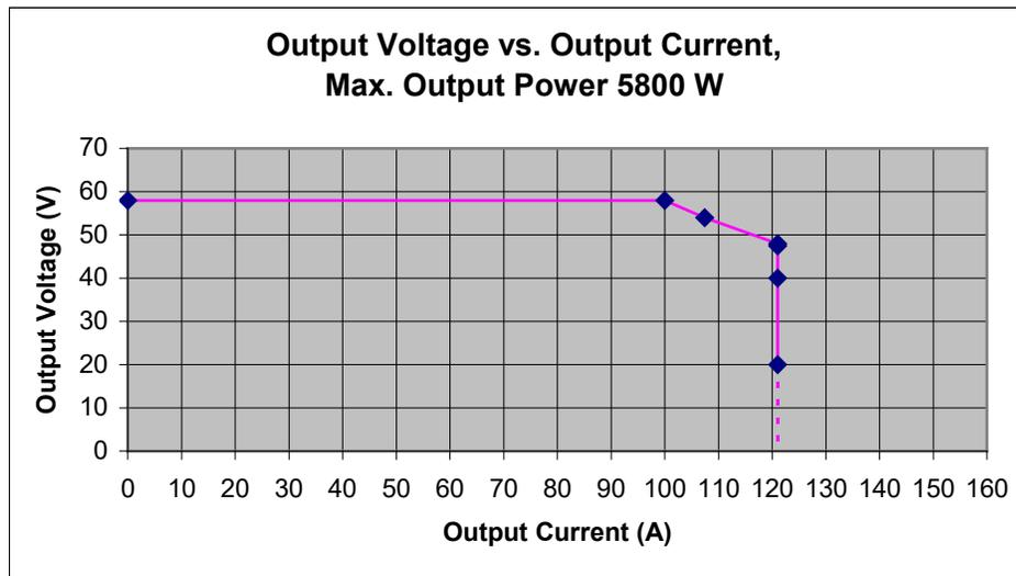
5.1.5 Power Derating Based on Input Voltage: The Rectifier Module power varies with changes in input voltage and output voltage. It uses an advanced power limitation method. The Rectifier Module can provide its maximum rated power (5800W) as long as the input voltage is within the range of 304 to 530 VAC (hysteresis is less than 3V). Below 304 VAC (and down to 260 VAC), the Rectifier Module will continue to operate normally but
