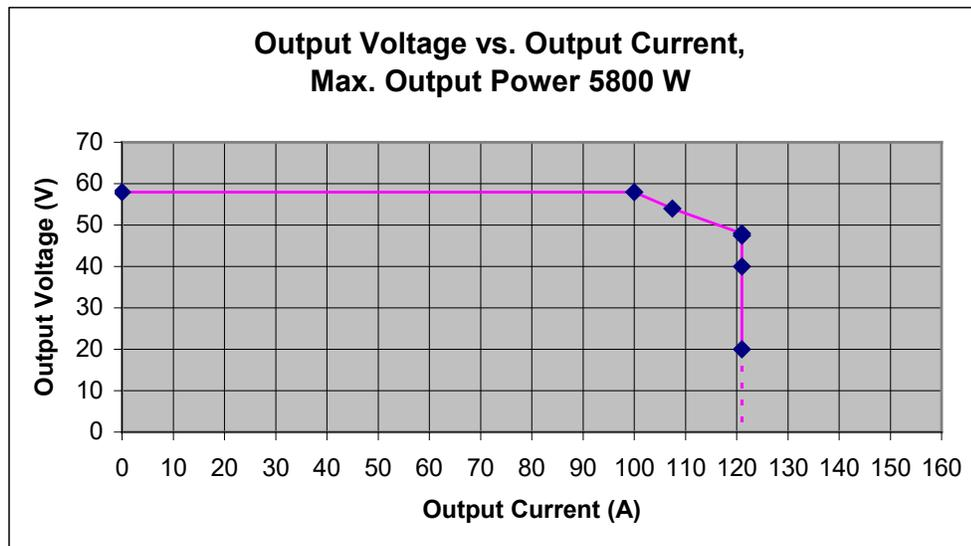
3.1.5 Power Derating Based on Input Voltage: The Rectifier Module power varies with changes in input voltage and output voltage. It uses an advanced power limitation method. The Rectifier Module can provide its maximum rated power (5800W) as long as the input voltage is within the range of 304 to 530 VAC (hysteresis is less
