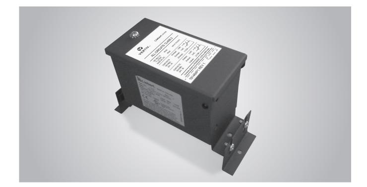
The Liebert® Liqui-Tect™ 410 (LT410) provides single-point detection of leaks. The point-detection sensor has two gold-plated sensing probes to prevent corrosion and to provide accurate readings. The LT410 constantly monitors for leaks, internal faults, and power failures and warns of any abnormal conditions. Mounting brackets allow for sensor height adjustment and leveling.
