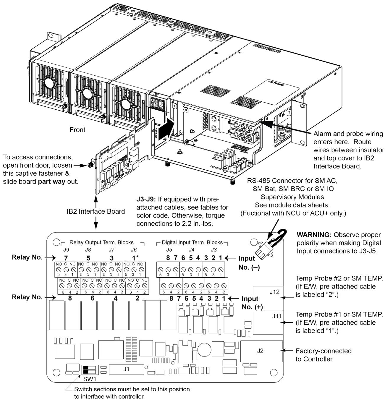
\* The relay assigned by the Controller to be the "Critical Summary" alarm (NCU or ACU+) or "Major Summary" alarm (SCU+) (relay 1 by default) will operate in the "Fail Safe Mode". Fail Safe Mode means the relay is de-energized during an alarm condition, opening the contacts between the C and NO terminals, and closing the contacts between the C and NC terminals.
