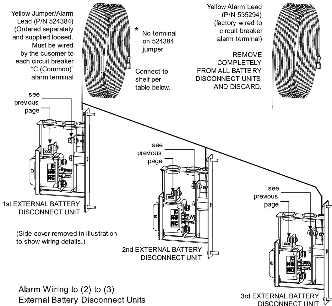
**Alarm Wiring to (2) to (3) External Battery Disconnect Units**
