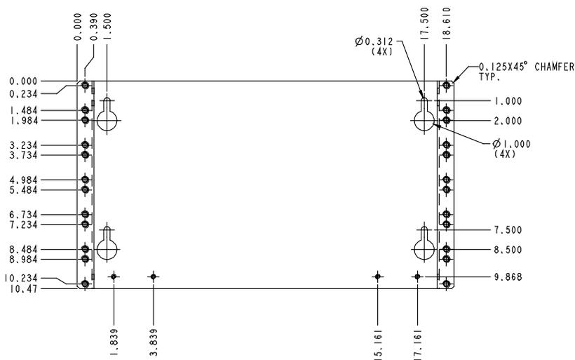
**Figure 5:** Horizontal Wall Mounting with P/N 552535
