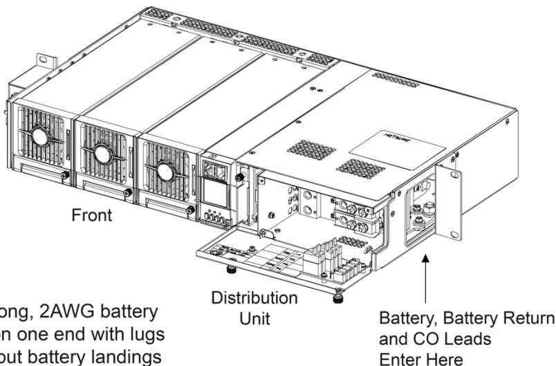
List 65 provides 3' long, 2AWG battery cables terminated on one end with lugs to connect to the input battery landings and on the other end with an Anderson connector.
