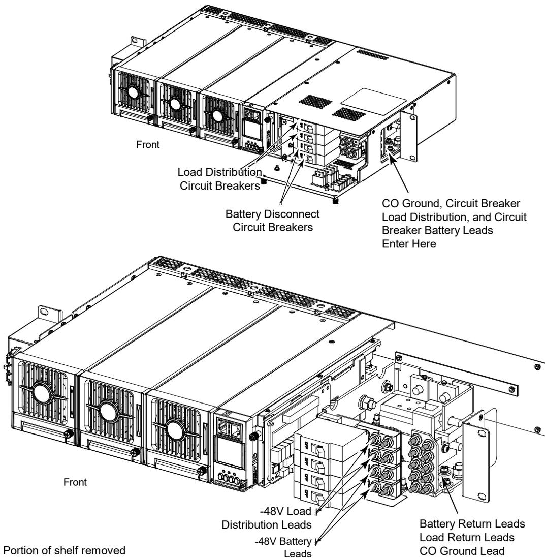
Portion of shelf removed in illustration for clarity. Leads are brought into side of shelf, and tools to secure lugs from front of shelf.
