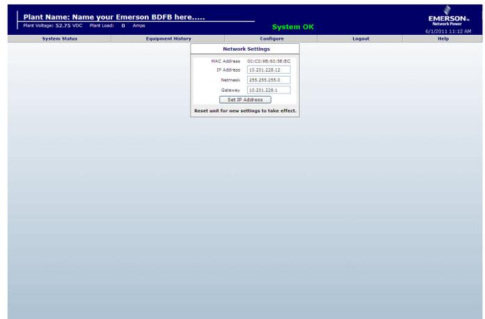
7. Enter the parameters issued by your IT department. When the required IP Address, Subnet Mask, and Gateway have been entered, click the **Set IP Address** button. **VERIFY WHAT YOU HAVE TYPED—IF IT IS ENTERED INCORRECTLY, YOU MAY NOT BE ABLE TO COMMUNICATE WITH THE BEC.**
