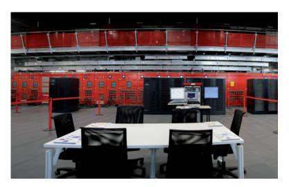
Al Load Simulator: A new addition enabling testing of variable Al load profiles, either pre-defined or specific to real cases applications. This equipment supports both design and validation testing, as well as customer demonstrations, ensuring UPS systems perform optimally under Al-driven loads and monitoring the main parameters for each scenario.
