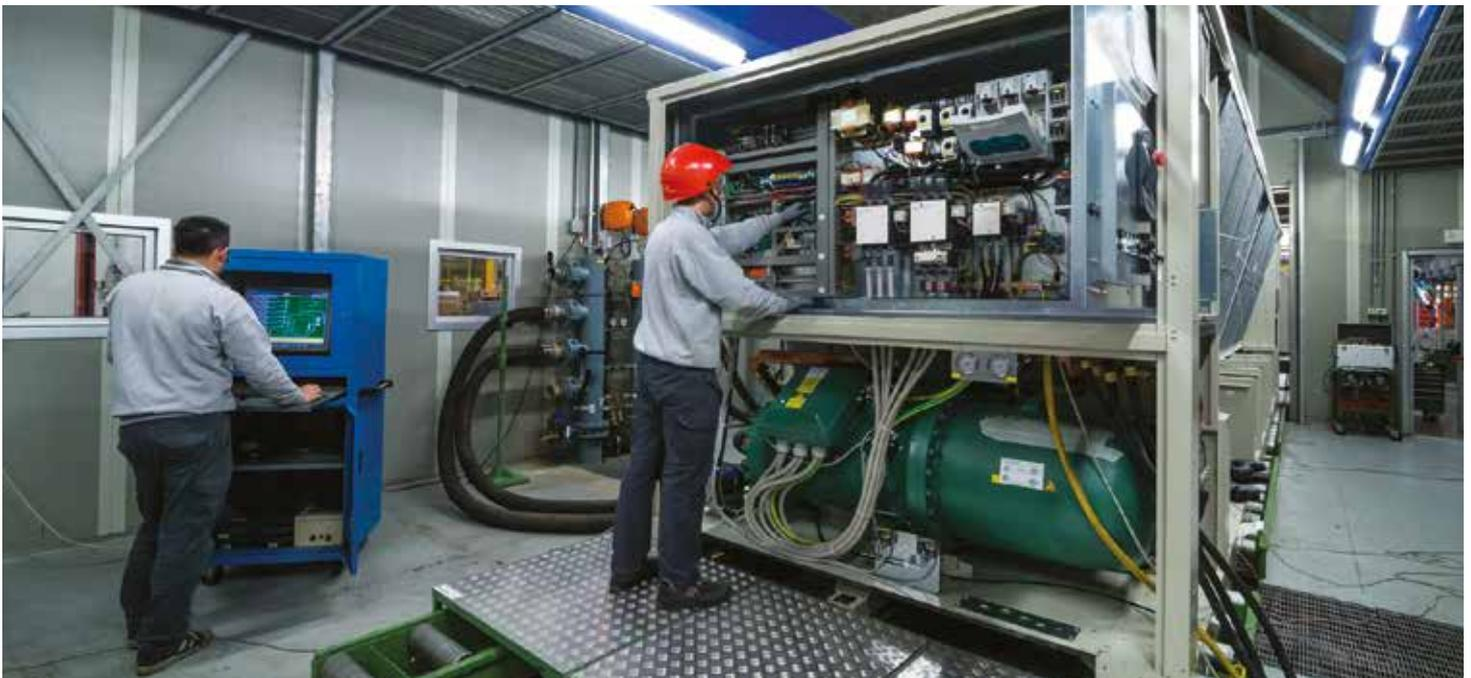
Chiller unit undergoing an end-of-line test
