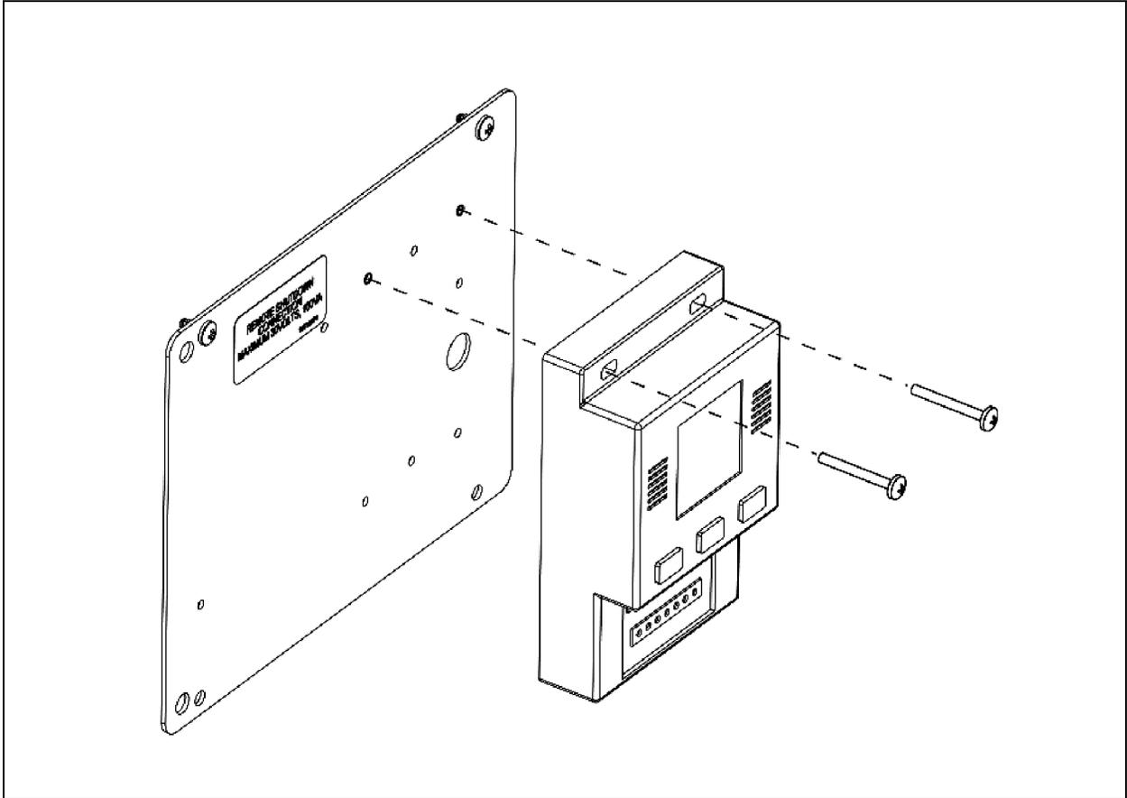
Figure 4.3 Attaching the Cable Tie Pad to the Temperature Sensor
