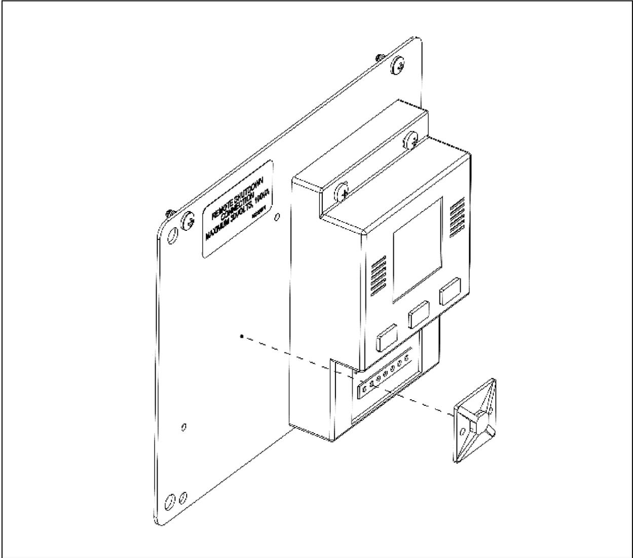
**NOTE:** Tie pad has rubber foam adhesive in the back.
