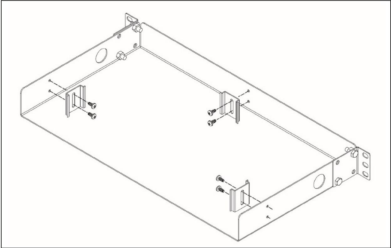
**NOTE:** Fix the rails DIN with the screws TPG PH PHL using a Philips head screwdriver.
