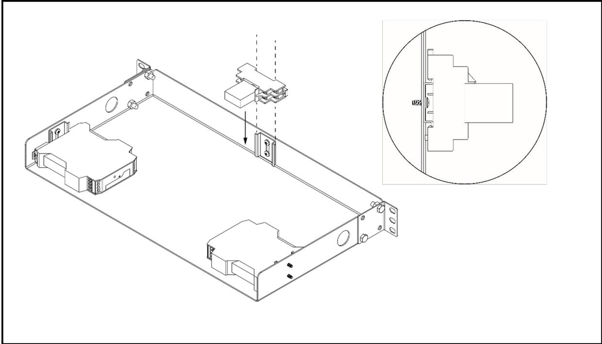
**NOTE:** The relay also must slide down through the DIN rail lugs until they contact the bracket of MCR Kit High Temperature Alarm. The relay should be fixed as shown in **Figure 4.7** above .
