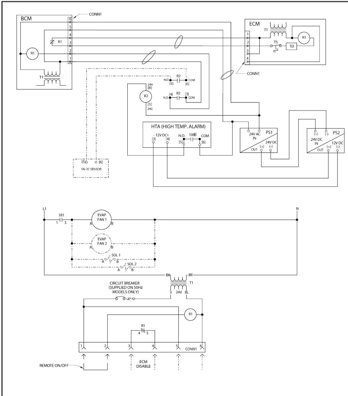
**NOTE:** Additional connections are made to this SN-3C from other sensors. In the RD MCR rack models, a ferrite bead is required in the electrical assembly. For more details, see **Figure 4.14** on the facing page and **Figure 4.15** on page 20 .
