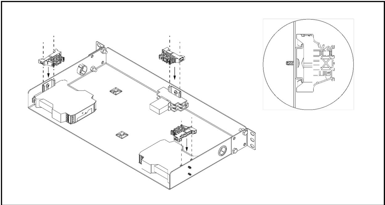
**NOTE:** In the same way as the converters and the relay, the retainers must slide down through the DIN rail lugs until they contact the converters and the relay. The retainers should be fixed as shown in **Figure 4.10** above .
