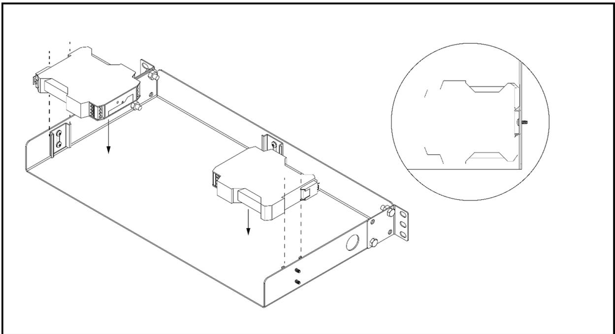
**NOTE:** The converters must slide down through the DIN rail lugs until they contact the bracket of Vertiv™ MCR Kit High Temperature Alarm. The converters should be fixed as shown in **Figure 4.6** on the previous page .
