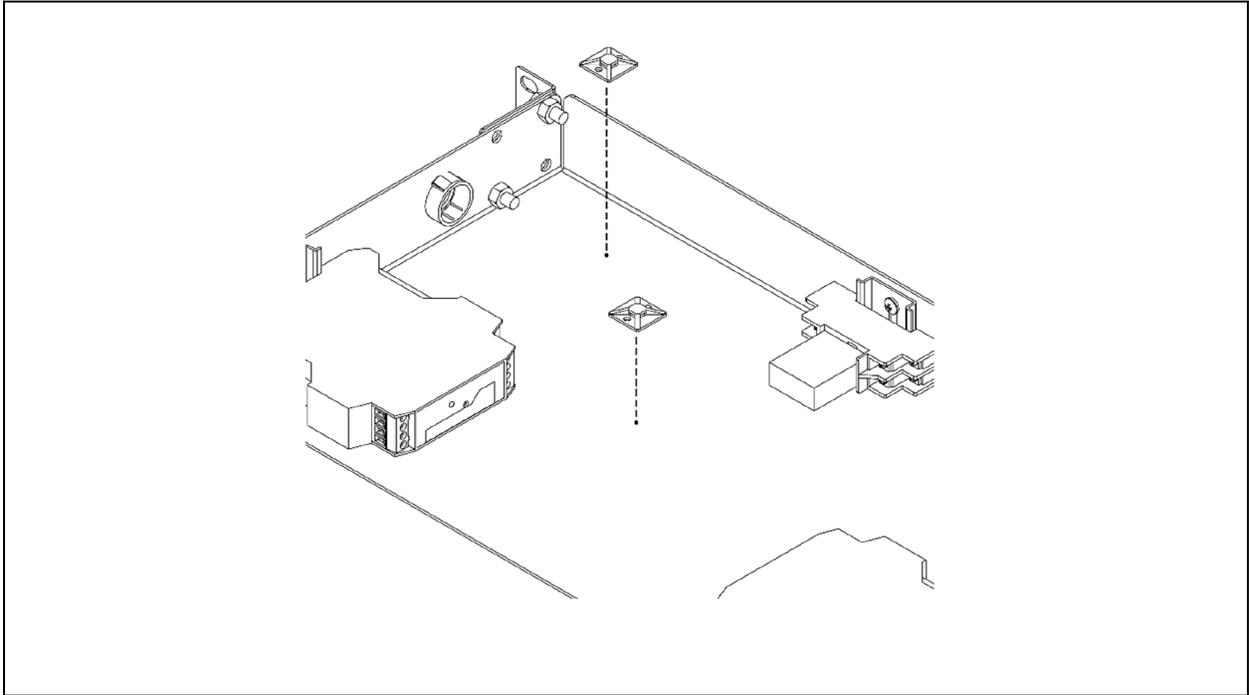
Figure 4.10 Attaching the Retainers to the Rail DIN
