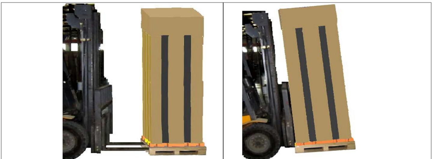
**Figure 2-3 Forklift Removal**
